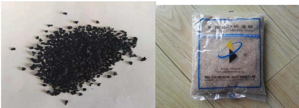
C: 1.5 mm rubber particles; D: Sand used in the test
