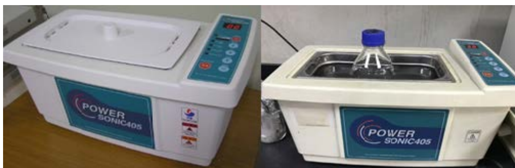
Fig. 1. Photograph of the lab-scale ultrasonic cleaner power sonic 405 (5 L) for water treatment.
