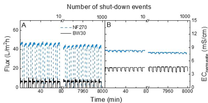
Fig. 1. Membrane performance (A) flux and (B) electrical conductivity of permeate as a function of time with 1000 shutdown events. Feed solution: 10 g/L NaCl with 1 mM NaHCO<sub>3</sub>, 24 ± 1°C. Each cycle: high-level solar irradiance 800 W/m<sup>2</sup> (namely 10 bar operating pressure) for 5 min dropping to zero (namely pump-off) for 3 min.
