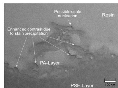
Fig. 4. TEM image of a RuO<sub>4</sub>-stained BW30 membrane cross-section. It shows a complex fold of the polyamide (PA)-layer nodules with dense stain precipitations present on the edges of the ridge-valley structures of the PA-layer as well as within the void spaces in the PA-layer.
