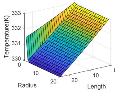
Fig. 3. Radial and longitudinal temperature profile for a  $T_{in} = 60^{\circ}\text{C}$ ,  $T_w = 70^{\circ}\text{C}$ ,  $v = 0.5$  m/s.
