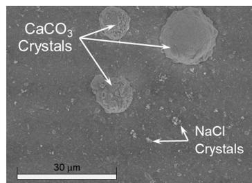
Fig. 2. SEM showed the CaCO<sub>3</sub> and NaCl crystals growth on the membrane; the identities of these crystals were verified by SEM-EDX.
