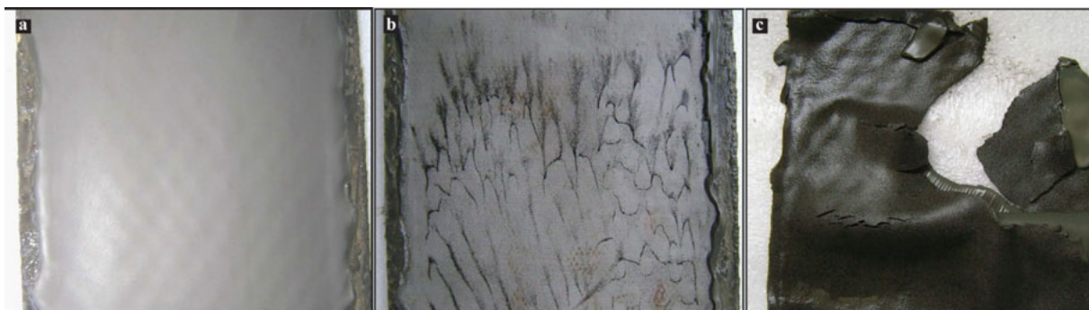
Fig. 7. Pictures of BPDDM: (a) before backwash; (b) after backwash; (c) cake layer right post-backwash.
