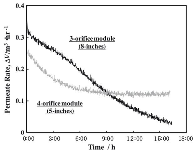
Fig. 5. Dependency of pure water's permeating rate into brine side against operation time on the number of the module orifice. Operation mode was PRO.
