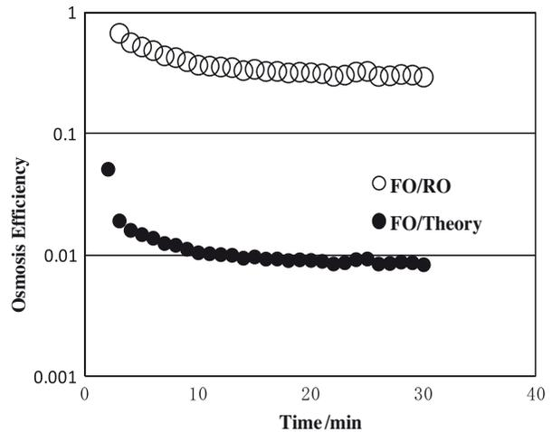
Fig. 8. Actual permeation flux ratio of PRO to RO mode, or to theoretically calculated PRO flux. The former one is denoted by open circle and the latter one by closed circle.
