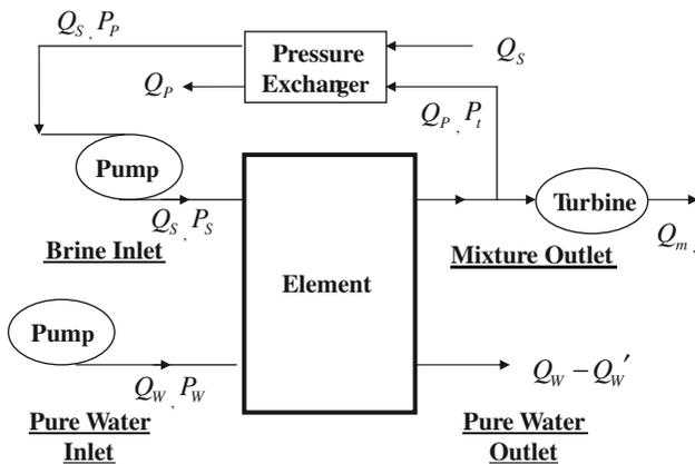
Fig. 2. Schematic diagram of bench scale plant. Symbols are summarized at the end of the text. Pure water outlet appeared only when 4-orifice module was employed.
