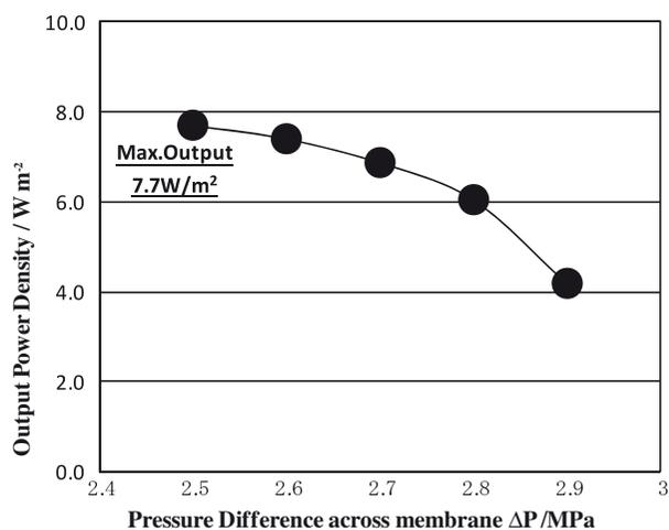
Fig. 10. Dependency of input and output power density on hydraulic pressure difference across membrane.
