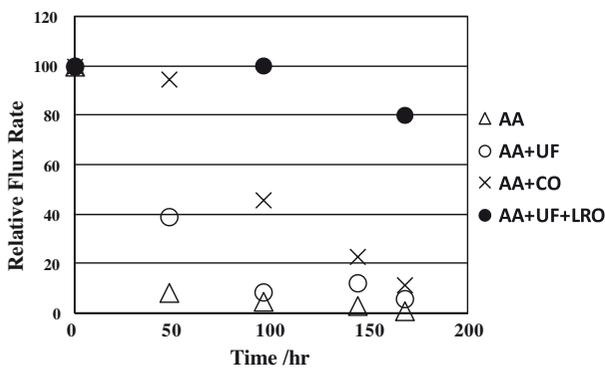
Fig. 7. Relative flux rate is shown compared with the flux value, as of the operation beginning, assumed as 100. AA; treated with anaerobic-aerobic activated sludge method AA+UF; treated with anaerobic-aerobic activated sludge method and then UF-unit AA+CO; treated with anaerobic-aerobic activated sludge method and then coagulation-sedimentation method with ozonation AA+UF+LRO; treated with anaerobic-aerobic activated sludge method, UF-unit and finally low pressure RO-unit.
