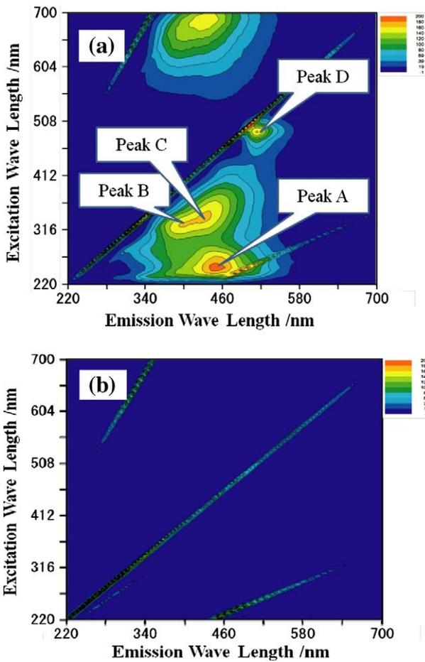
Fig. 6. EEM analysis result of (a) the pure water sample after treatment with the UF membranes and (b) concentrated brine coming from the SWRO.
