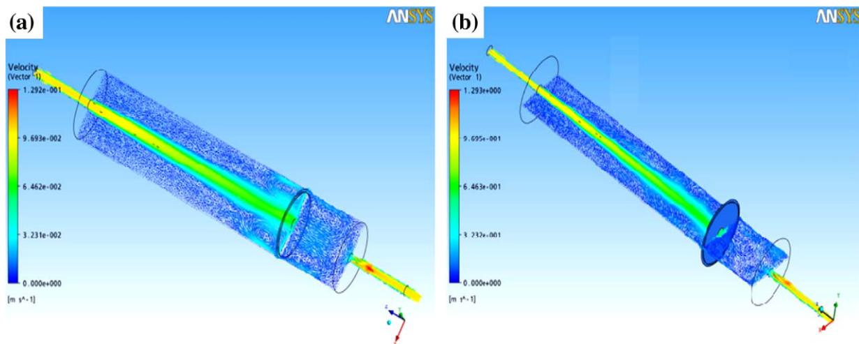
Fig. 9. Simulation results of brine flow inside the SWRO element at PRO operation. Pressure drop inside element is zero (a) and several hundred kPa (b).
