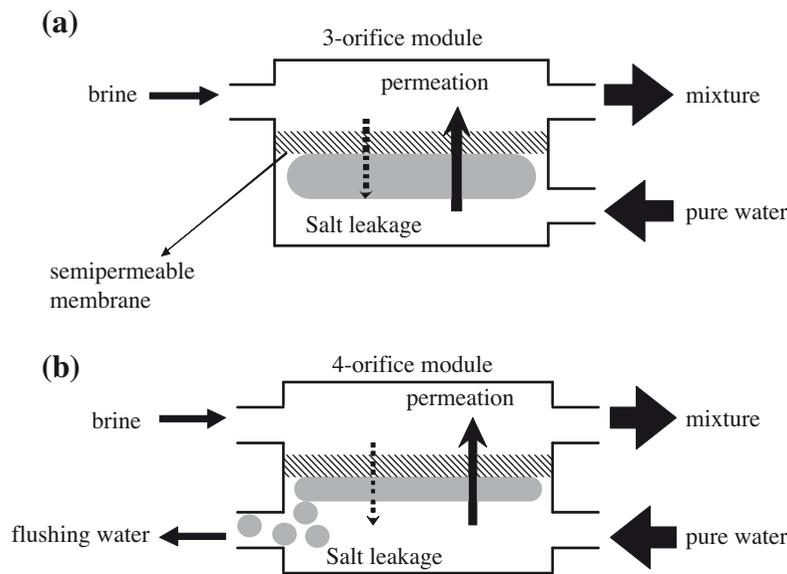
Fig. 4. Schematic picture of 4-orifice module in comparison with conventional 3-orifice module. If using 3-orifice module, salt leaks from brine side to pure water side and accumulates at the membrane surface as described by the shadowed area.
