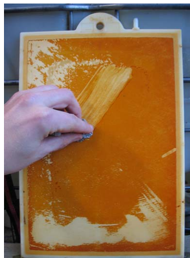
Fig. 5. Cake layer deposit composed of soluble and colloidal material coagulated by \text{FeCl}_2 .
