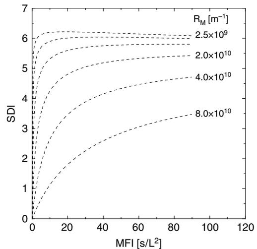
Fig. 2. The mathematical relation between SDI and MFI influenced by the membrane resistance ( $0.25 \times 10^{10}$ – $8.0 \times 10^{10} \text{ m}^{-1}$ ). Reference parameters were assumed: membrane area ( $A_M$ )  $13.8 \times 10^{-4} \text{ m}^2$ , temperature  $20^\circ\text{C}$  and applied pressure (dP) 207 kPa.
