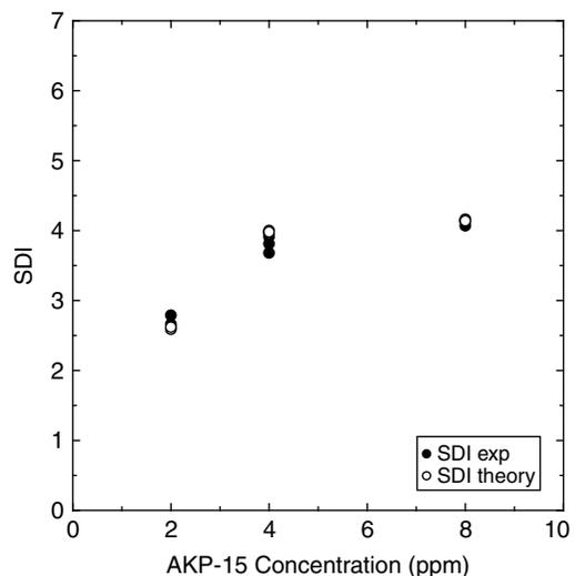
Fig. 3. Theoretical and experimental SDI results for different particle concentrations (2, 4 and 8 ppm). Feed solutions contained  $\alpha$ -Alumina particles (AKP-15) with  $0.6 \mu\text{m}$  size. The filtration experiments were carried out using cellulose acetate membranes M6.
