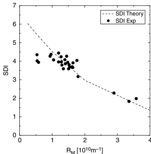
Fig. 4. SDI experimental and theoretical results for different membrane resistance materials and manufactures. The experiments carried out using particles concentration 4 ppm of AKP-15 under pressure 207 kPa.
