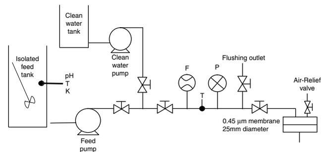
Fig. 1. Flowsheet of the SDI setup. Feed tank and clean water tank are shown. pH, Temperature ( $T$ ) and conductivity ( $K$ ) are measured in the feed tank as well as in the feed line. Pressure ( $P$ ), flow rate ( $F$ ) and temperature ( $T$ ) are measured in the feed line. Valves are controlled using software using ViCA.
