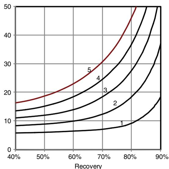
Fig. 2. The pressures determined inversely from Eq. (10) for a constant average permeate flux of  $6.89 \times 10^{-6}$  m s<sup>-1</sup> in a RO with feed salt concentrations of: (1). 2500 mg l<sup>-1</sup>, (2). 5000 mg l<sup>-1</sup>, (3). 7500 mg l<sup>-1</sup>, (4). 10,000 mg l<sup>-1</sup>, and (5). 12,500 mg l<sup>-1</sup>.
