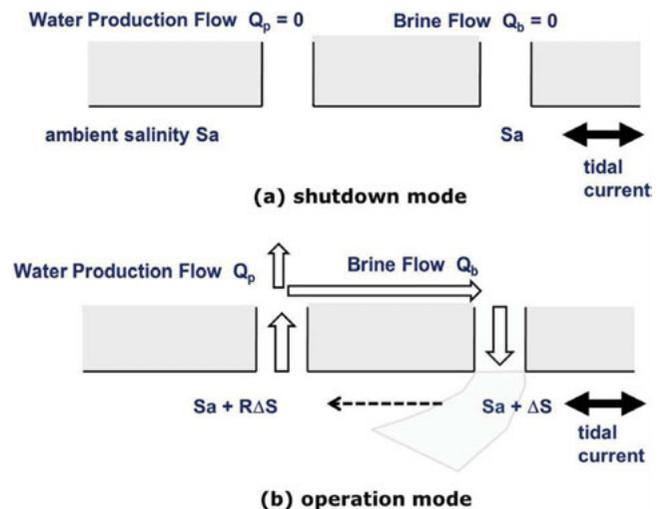
Fig. 3. Recirculation of a desalination plant.
