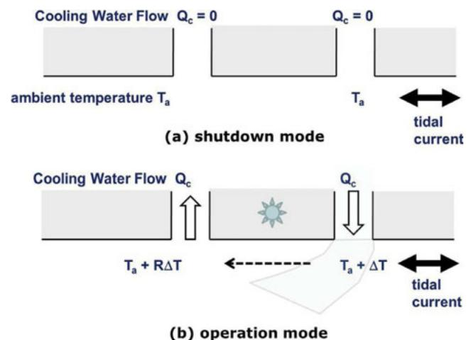
Fig. 1. Recirculation of a thermal power plant.
