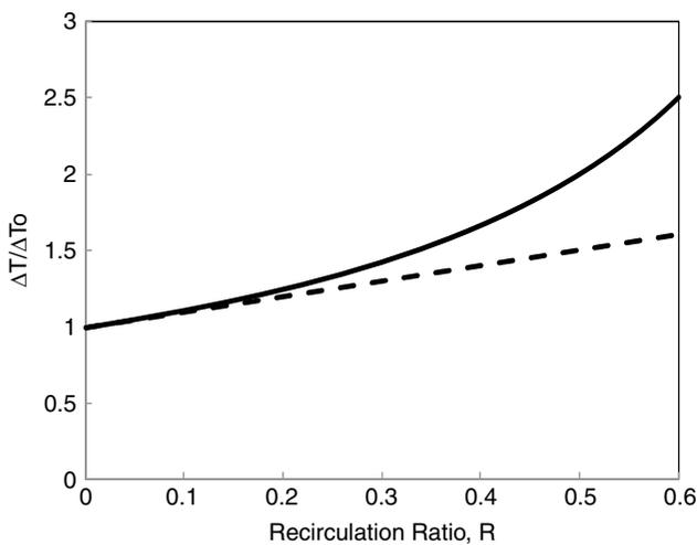
Fig. 2. Relationship between the non-dimensional temperature increase and recirculation ratio for a thermal power plant.
