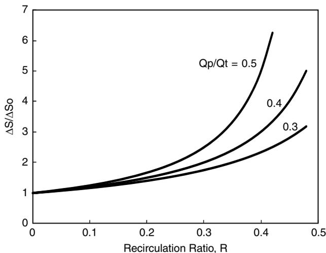
Fig. 4. Relationship between the non-dimensional salinity rise and recirculation ratio for a desalination plant.
