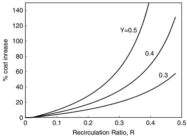
Fig. 5. Relationship between the % cost increase and recirculation ratio for a desalination plant.
