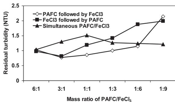
Fig. 3. Effects of dosage mass of the combined PAFC/ $\text{FeCl}_3$  on the residual turbidity removal.
