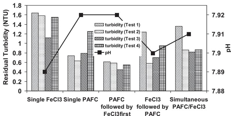
Fig. 2. Effect of dosing order of the combined  $\text{FeCl}_3$ /PAFC on turbidity removal efficiency.
