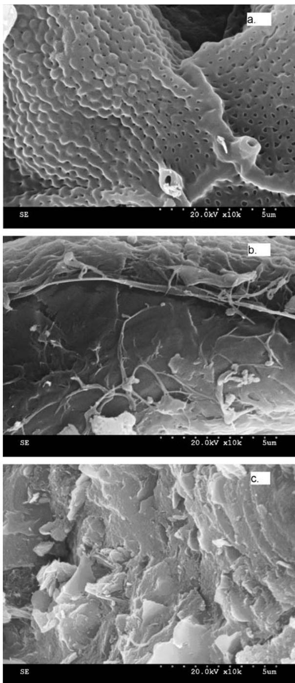
Fig. 6. SEMs for the flocs formed using different coagulants/coagulant aid, with the magnification of 10,000. (a) Single  $\text{FeCl}_3$ , (b) single PAFC, and (c) combined PAFC/ $\text{FeCl}_3$ .
