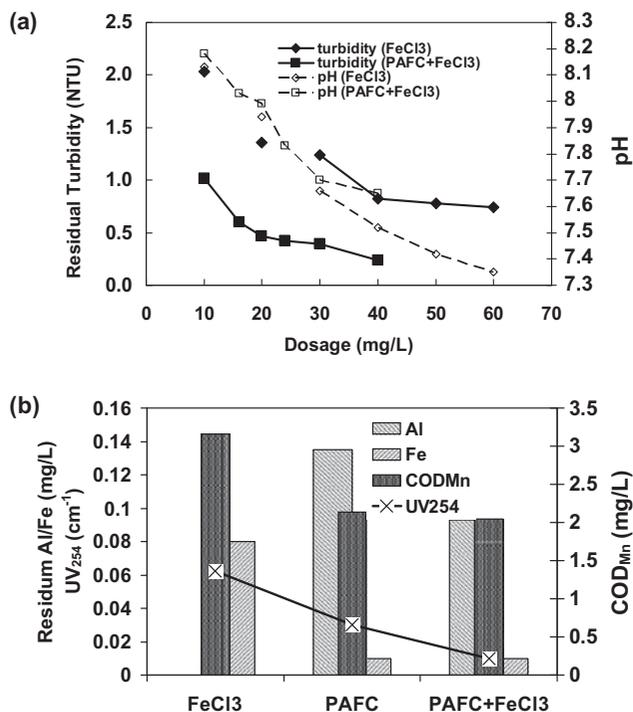
Fig. 5. Coagulation optimization by integrating combined coagulant dosage, order, ratio, and time interval using single FeCl<sub>3</sub> and combined coagulants FeCl<sub>3</sub>/PAFC with the total dosage of 20 mg/L. (a) Change of residual turbidity for different amount of coagulant dosage, (b) and (c) Residual Fe and Al concentration and UV<sub>254</sub>.
