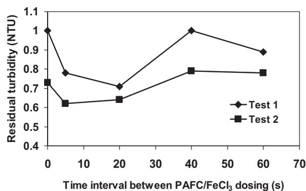
Fig. 4. Effects of dosing interval of the combined PAFC/ $\text{FeCl}_3$  on turbidity removal.
