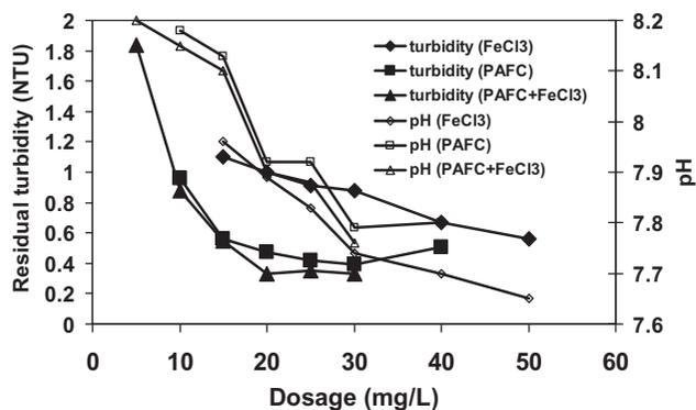
Fig. 1. The comparison of single  $\text{FeCl}_3$ , single PAFC, and combined PAFC/  $\text{FeCl}_3$  on turbidity removal efficiency.
