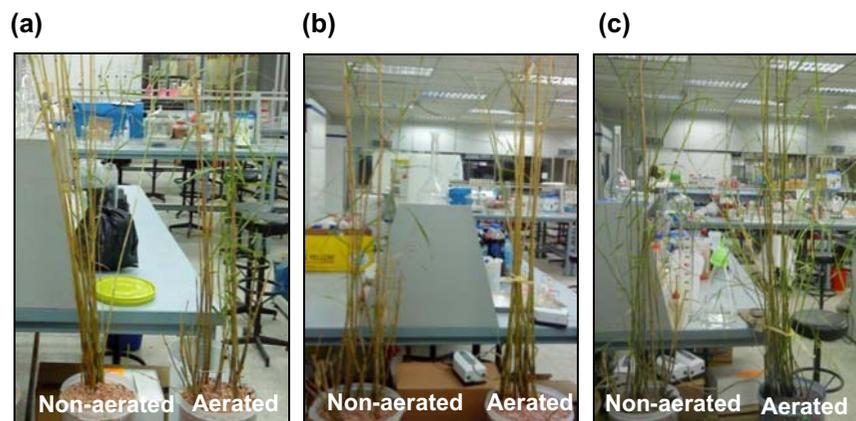
Fig. 2. Observation of emergent plants: (a) first day of transplantation, (b) one week, and (c) one month after the addition of RB5-containing wastewater.
