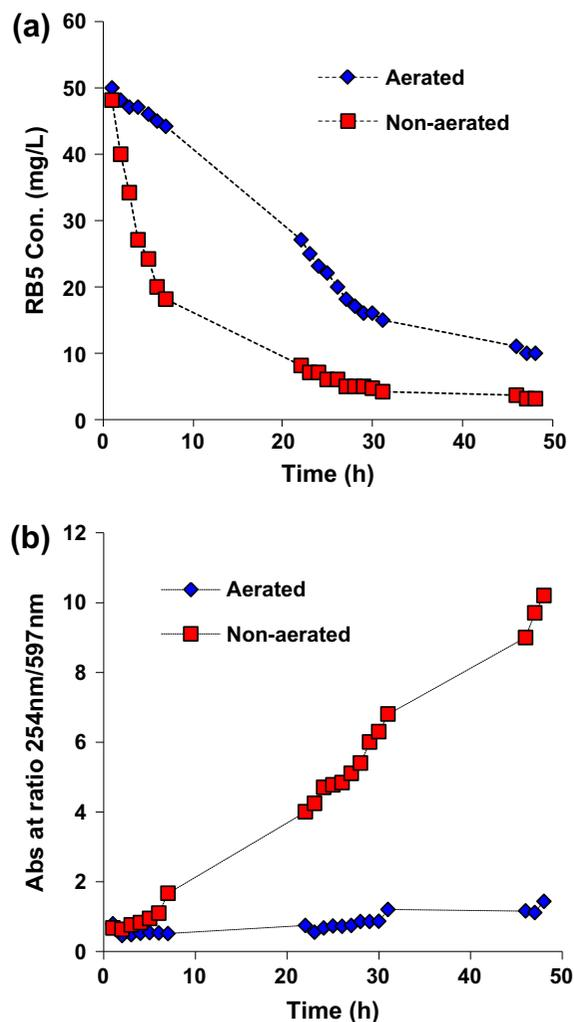
Fig. 5. Color (a) and aromatic amines (b) monitoring of the water samples collected from UFCW reactors.
