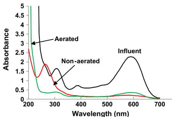
Fig. 4. UV-vis spectrum analysis of the water samples collected from UFCW reactors.
