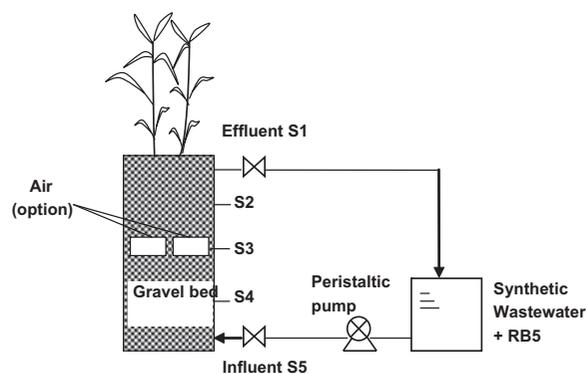
Fig. 1. Schematic diagram of a recirculated UFCW reactor.
