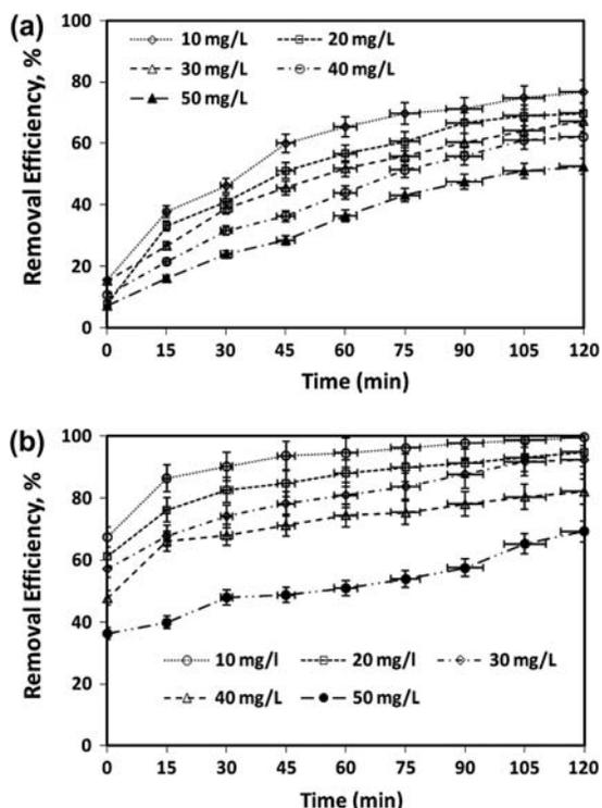
Fig. 4. Effect of initial Cr(VI) concentration on the removal of Cr(VI) in purging of (a) oxygen and (b) nitrogen gas (pH=4, TiO<sub>2</sub>=1 g/L).
