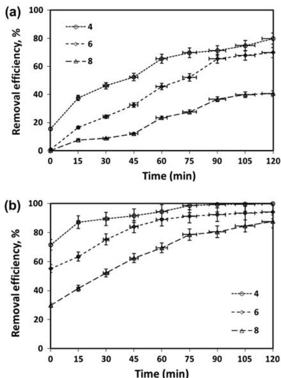
Fig. 2. Effect of pH on the removal of Cr(VI) in purging of (a) oxygen and (b) nitrogen gas (TiO<sub>2</sub> = 1 g/L, Cr(VI) = 10 mg/L).
