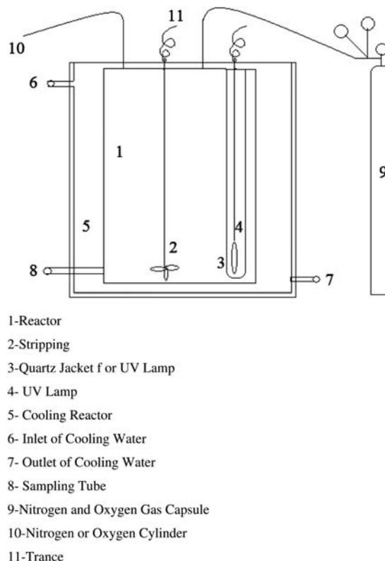
Fig. 1. A schematic diagram of the experimental setup for photocatalysis.
