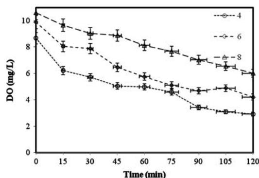
Fig. 3. Variation of the concentration of dissolved oxygen at different pH during the photocatalytic reaction in purging of oxygen.
