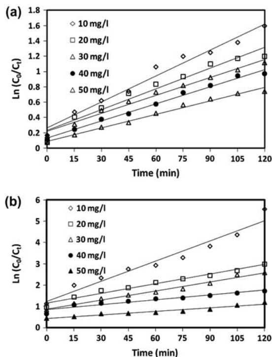
Fig. 5. First-order kinetic model for Cr(VI) removal in purging of (a) oxygen and (b) nitrogen gas (pH=4, TiO<sub>2</sub>=1 g/L).
