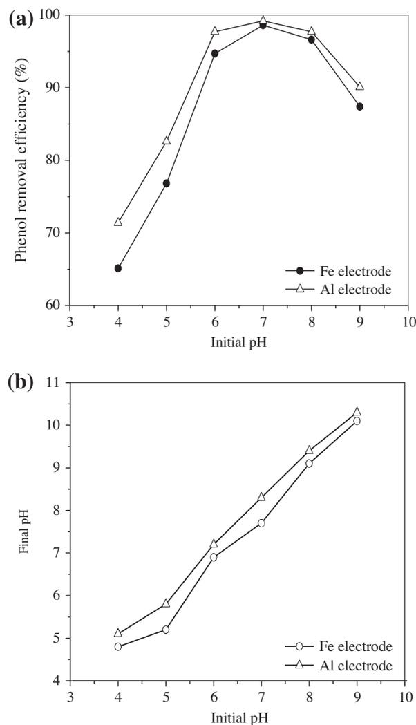
Fig. 1. (a) Effect of initial pH on the removal of phenol from aqueous solutions and (b) changes in initial pHs (conditions: Current density of  $40 \text{A}/\text{m}^2$ , initial phenol concentration of  $50 \text{mg}/\text{L}$ , and conductivity of  $1,200 \mu\text{S}/\text{cm}$ ).
