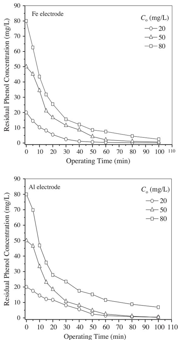
Fig. 3. Effect of initial phenol concentration on the removal of phenol from aqueous solutions (conditions: Current density of  $40 \text{ A/m}^2$ , initial pH 7, and conductivity of  $1,200 \text{ }\mu\text{S/cm}$ ).
