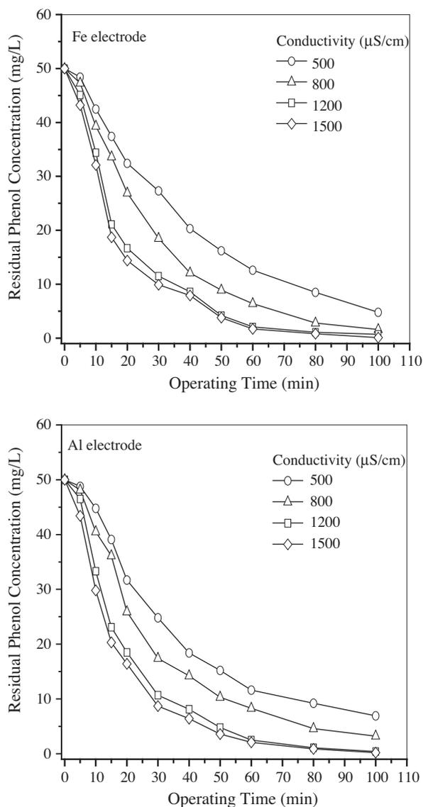
Fig. 4. Effect of conductivity on the removal of phenol from aqueous solutions (conditions: Current density of  $40 \text{ A/m}^2$ , initial pH 7, and initial phenol concentration of  $50 \text{ mg/L}$ ).
