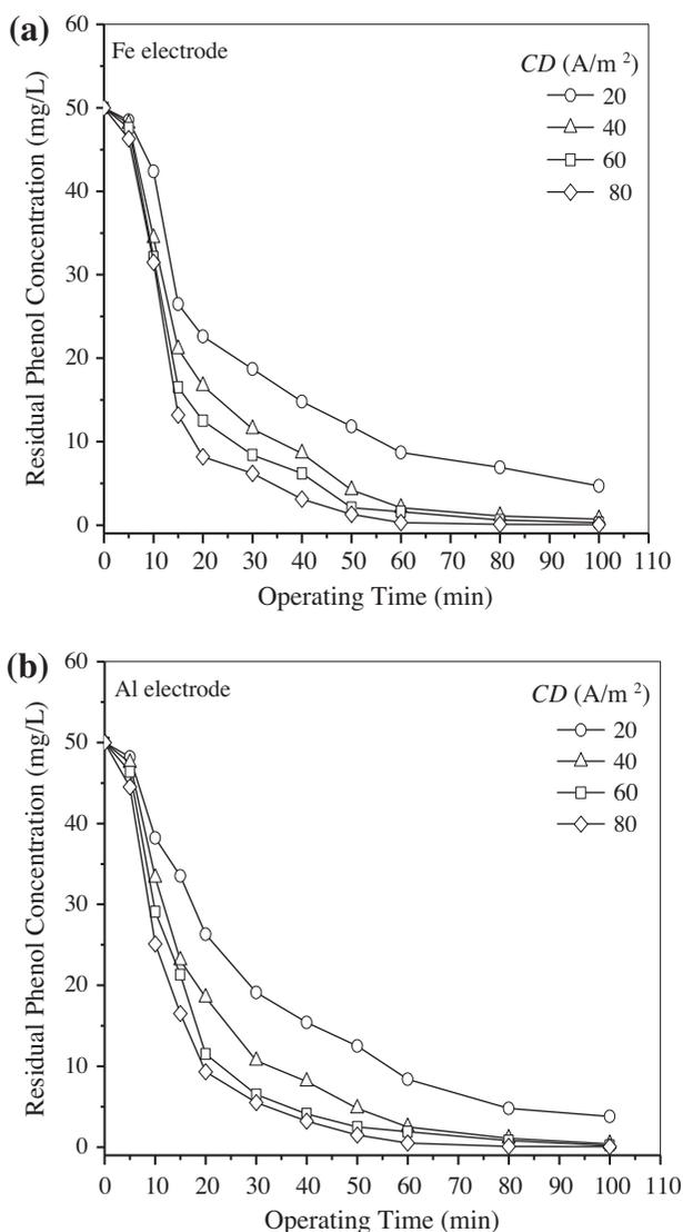
Fig. 2. Effect of current density on the removal of phenol from aqueous solutions (conditions: initial phenol concentration of 50 mg/L, initial pH 7, and conductivity of 1,200  $\mu\text{S}/\text{cm}$ ).
