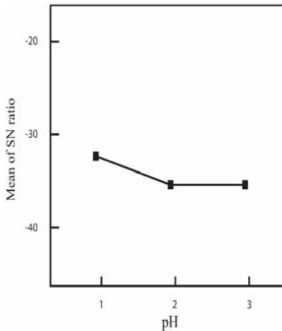
Fig. 3. The effect of pH on the S/N ratio in the removal with pistachionut shell. ( $T = 20\text{ }^{\circ}\text{C}$ , adsorbent particle size =  $0.025 < x < 0.5$ ,  $C_i = 50\text{ ppm}$ , agitation speed =  $150\text{ rpm}$ )
