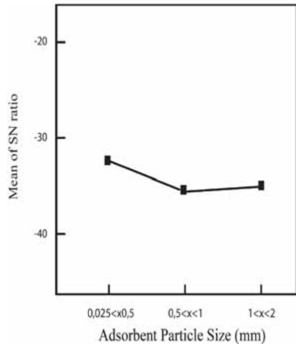
Fig. 4. The effect of adsorbent particle size on the S/N ratio in the removal with pistachionut shell. ( $T = 20\text{ }^{\circ}\text{C}$ , adsorbent concentration =  $0.3\text{ g}$ ,  $C_i = 50\text{ ppm}$ , agitation speed =  $150\text{ rpm}$ ).
