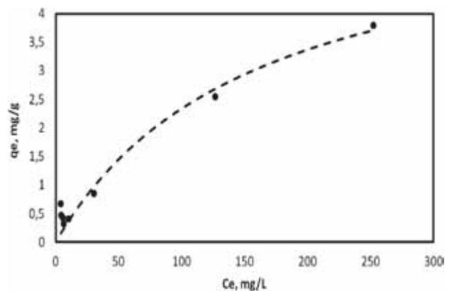
Fig. 11. Langmuir plots for the adsorption of Remazol Rot RB dye onto pistachionut shell.
