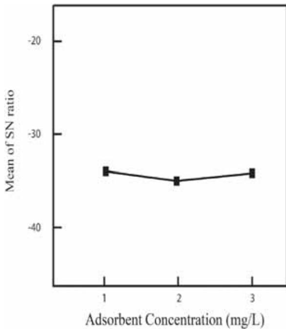
Fig. 6. The effect of adsorbent concentration on the S/N ratio in the removal with pistachionut shell. ( $T = 20\text{ }^{\circ}\text{C}$ ,  $\text{pH} = 2$ , contact time = 10 min,  $C_i = 50\text{ ppm}$ , agitation speed = 150 rpm).
