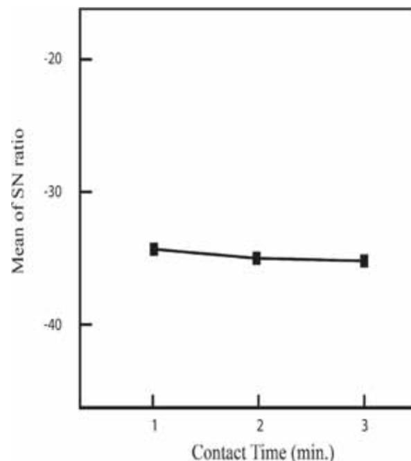
Fig. 5. The effect of contact time on the S/N ratio in the removal with pistachionut shell ( $T = 20\text{ }^{\circ}\text{C}$ , pH = 2, adsorbent concentration =  $0.3\text{ g}$ ,  $C_i = 50\text{ ppm}$ , agitation speed =  $150\text{ rpm}$ ).
