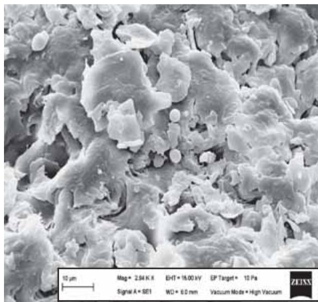
Fig. 1. SEM micrograph of the pistachio nut shells with Remazol Rot RB adsorbed.
