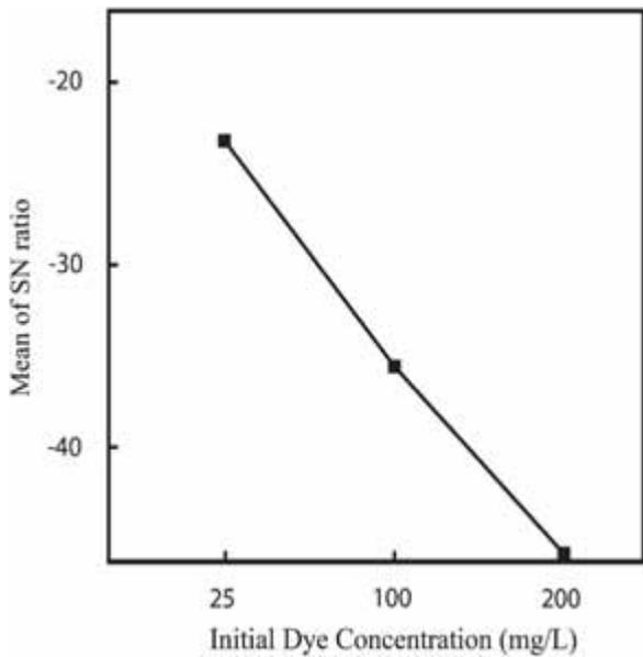
Fig. 9. The effect of initial dye concentration on the S/N ratio in the removal with pistachionut shell\*. ( $T = 20\text{ }^{\circ}\text{C}$ ,  $\text{pH} = 2$ , contact time = 10 min, agitation speed = 150 rpm, adsorbent particulate size =  $0.025 < x < 0.5$ ).
