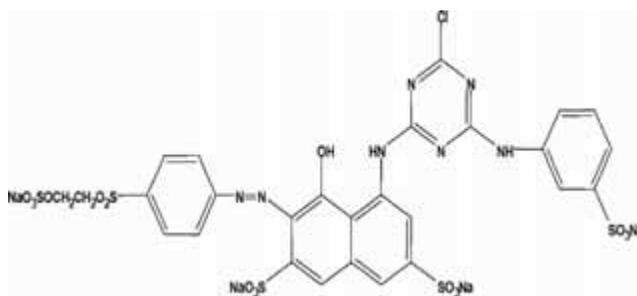
Fig. 2. The chemical structure of Remazol Rot RB (C.I. Reactive Red 198).
