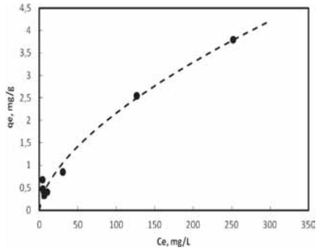
Fig. 10. Freundlich plots for the adsorption of Remazol Rot RB dye onto pistachionut shell.
