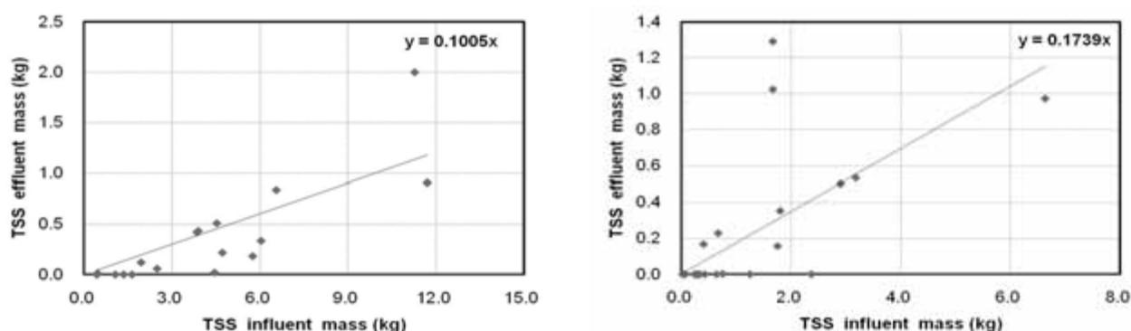
Fig. 3. ROL plot for use in calculating efficiency for TSS in monitoring sites. (a) Site 1 (Slope = 0.1005). (b) Site 1 (Slope = 0.1739).
