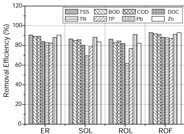
Fig. 5. Comparison of removal efficiencies for combined sites using the four methods.
