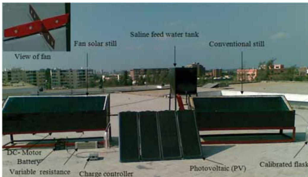
Fig. 1. Photograph of experimental setup.
