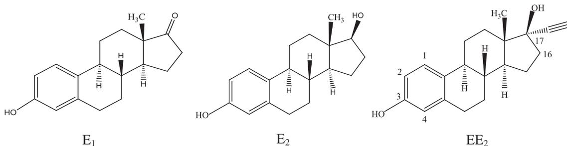
Fig. 1. The structural formulas of the three estrogens.
