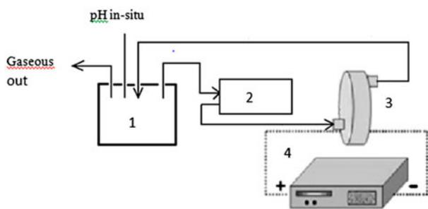
Fig. 1. Experimental setup: (1) back of solution, (2) pump, (3) electrochemical cell, and (4) power supply.
