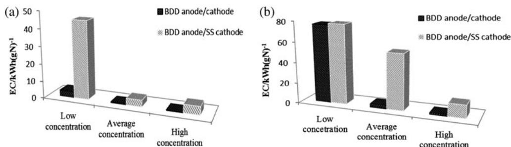
Fig. 8. Histograms of EC ( $\text{kWh}(\text{gN})^{-1}$ ) in case of nitrate (a) and nitrite (b) reduction at BDD anode/cathode and at BDD anode/SS cathode.
