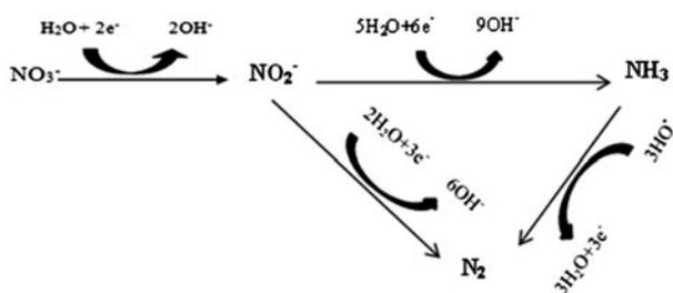
Fig. 6. Mechanism of electro-reduction in nitrate at BDD anode/cathode.
