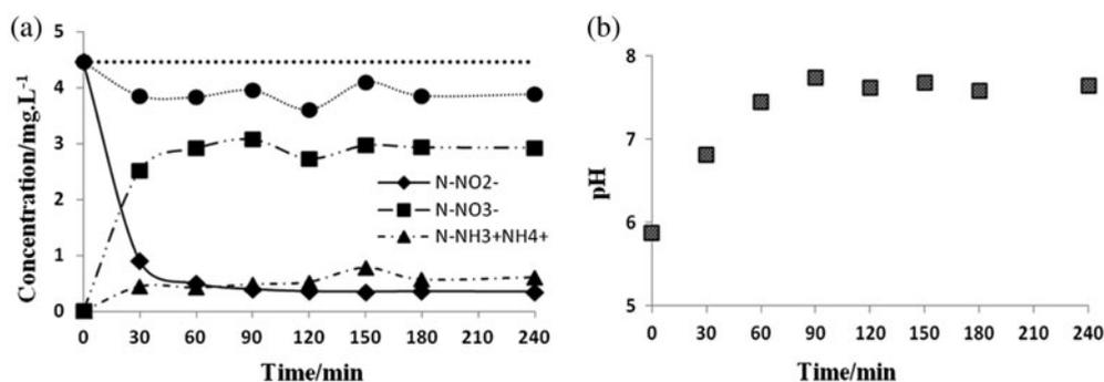
Fig. 7. Concentrations of nitrite removal ( $\blacklozenge$  N-NO<sub>2</sub><sup>-</sup> by-products formed; ( $\blacksquare$ ) N-NO<sub>3</sub><sup>-</sup>, ( $\blacktriangle$ ) N-NH<sub>3</sub>, and ( $\bullet$ ) total nitrogen (a) during the electrolysis of 4.46 mg L<sup>-1</sup> pH evolution with electro-reduction time (b). Experimental conditions: BDD anode, SS cathode;  $j = 40$  mA cm<sup>-2</sup>; supporting electrolyte Na<sub>2</sub>SO<sub>4</sub> (0.1 M); pH<sub>0</sub> = 6.0 ± 0.2.
