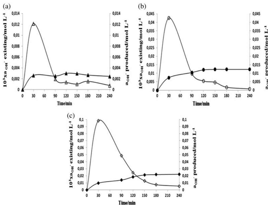
Fig. 3. Comparison between the quantity produced (open symbols) and existing (solid symbols) of ion hydroxyl with electrolysis times during the electro-reduction in:  $65 \text{ mg L}^{-1}$  (a),  $250 \text{ mg L}^{-1}$  (b), and  $500 \text{ mg L}^{-1}$  (c) of  $\text{N-NO}_3^-$  at BDD anode/cathode.
