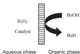
Fig. 2. Partial oxidation of BzOH to BzH by a membrane non-dispersive L–L reactor.
