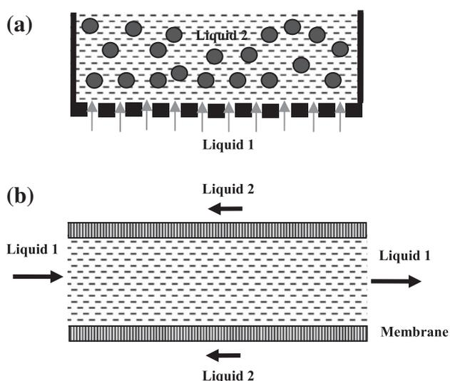
Fig. 1. Schematic diagram of membrane liquid-liquid reactors. (a) Membrane-dispersive reactor. (b) Membrane non-disperse reactor.
