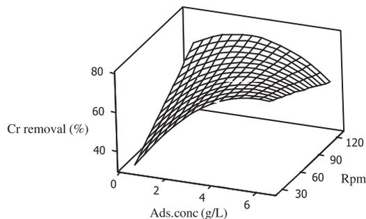
Fig. 12. Effect of RPM and adsorbent concentration on chromium(VI) removal.
