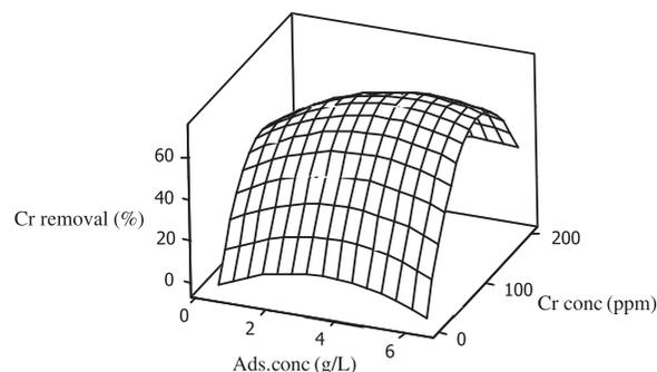
Fig. 11. Effect of chromium concentration and adsorbent concentration on chromium(VI) removal.
