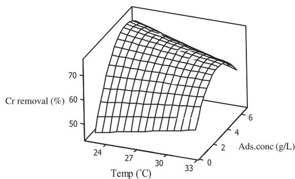
Fig. 8. Effect of adsorbent concentration and temperature on chromium(VI) removal.
