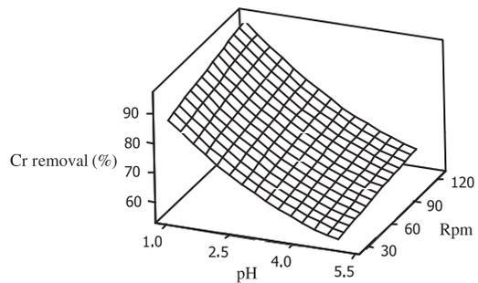
Fig. 7. Effect of RPM and pH on chromium(VI) removal.
