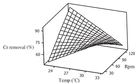
Fig. 10. Effect of RPM and temperature on chromium(VI) removal.
