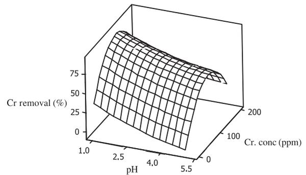
Fig. 6. Effect of chromium concentration and pH on chromium(VI) removal.
