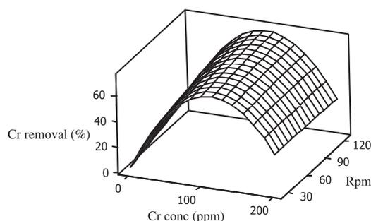
Fig. 13. Effect of RPM and chromium concentration on chromium(VI) removal.
