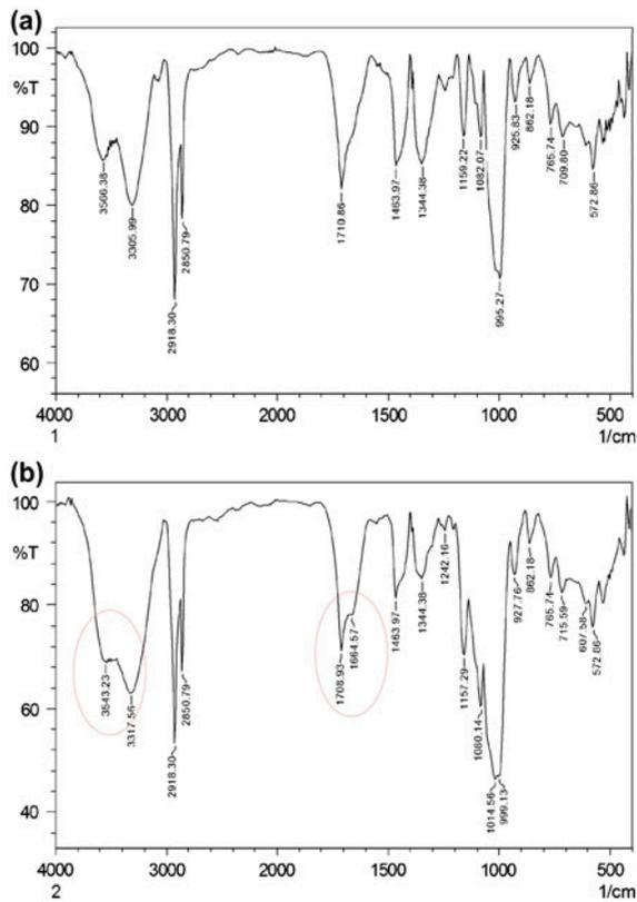
Fig. 3. FTIR spectra of raw (a) and chromium loaded (b) mango seed powder.
