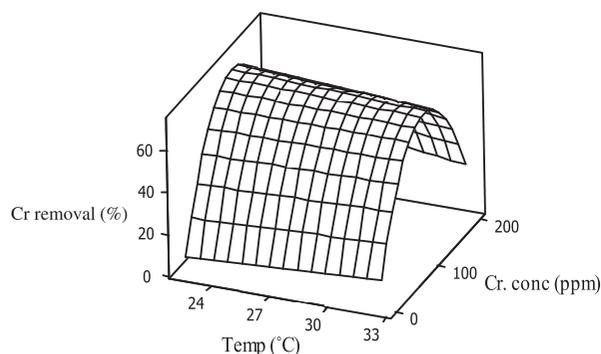
Fig. 9. Effect of chromium concentration and temperature on chromium(VI) removal.
