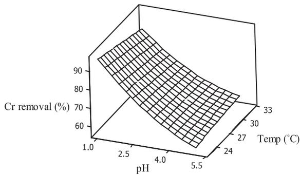
Fig. 4. Effect of pH and temperature on chromium(VI) removal.
