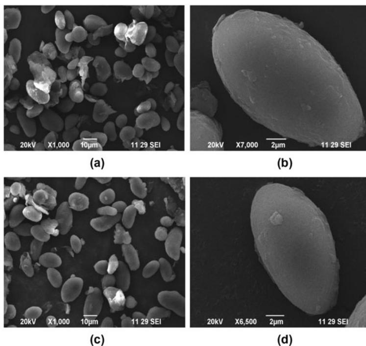
Fig. 2. SEM images of raw adsorbent (a), (b) and chromium-loaded adsorbent (c), (d).
