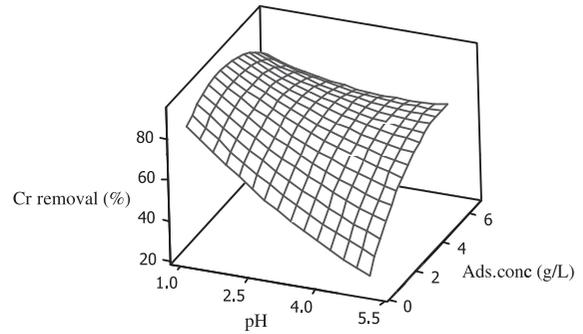
Fig. 5. Effect of adsorbent concentration and pH on chromium(VI) removal.
