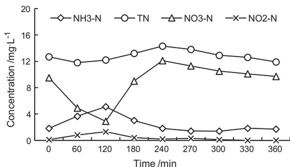
Fig. 7. Temporal variations of nitrogen conformation within one operation cycle under C operating mode.
