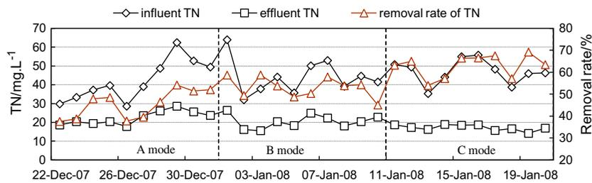
Fig. 5. The comparison of TN removal performance under low-temperature and different operation modes.
