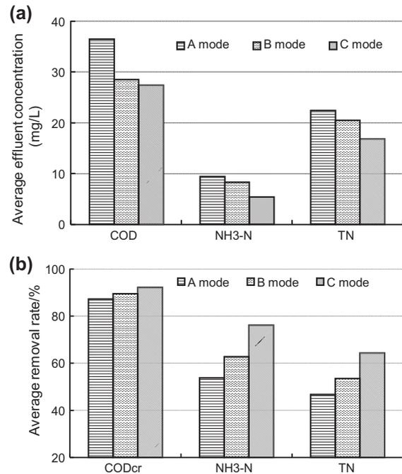
Fig. 6. (a) Average effluent concentration and (b) average removal rate of COD<sub>cr</sub>, NH<sub>3</sub>-N, and TN under three different low-temperature operating modes.
