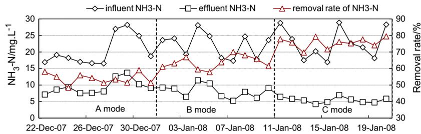
Fig. 4. The comparison of NH<sub>3</sub>-N removal performance under low-temperature and different operation modes.
