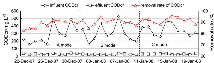
Fig. 3. The comparison of COD removal performance under low-temperature and different operation modes.
