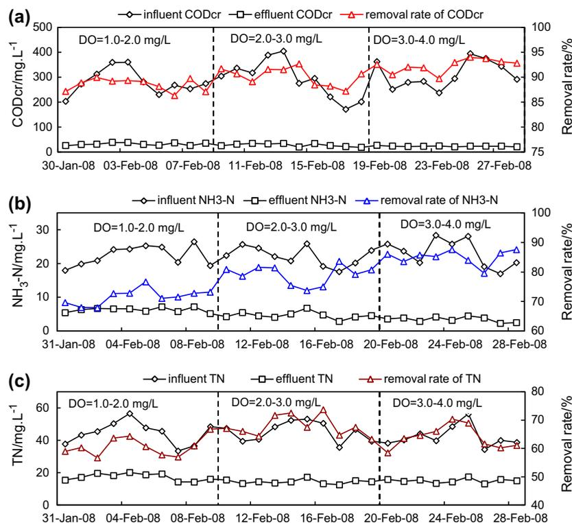
Fig. 8. (a) COD<sub>Cr</sub>, (b) NH<sub>3</sub>-N, and (c) TN removal performance under conditions of different DO levels.
