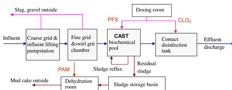
Fig. 1. Flow chart of treatment process of CAST (PFS: Poly Ferric Sulfate; PAM: Polyacrylamide;  $\text{ClO}_2$ : chlorine dioxide). Notes: PFS is used as reagent dosing for the chemical phosphorus removal, the dosage point lies in the center of biological selection zone of CAST biochemical pool;  $\text{ClO}_2$  is used reagent dosing for the disinfection of contact tank; PAM is the organic polymer flocculant used for the sludge dewatering, the dosage is 4 kg (PAM) powder/ton dry sludge.
