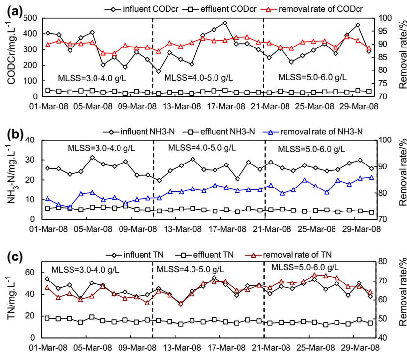
Fig. 9. (a) COD<sub>Cr</sub>, (b) NH<sub>3</sub>-N, and (c) TN removal performance under conditions of different MLSS levels.
