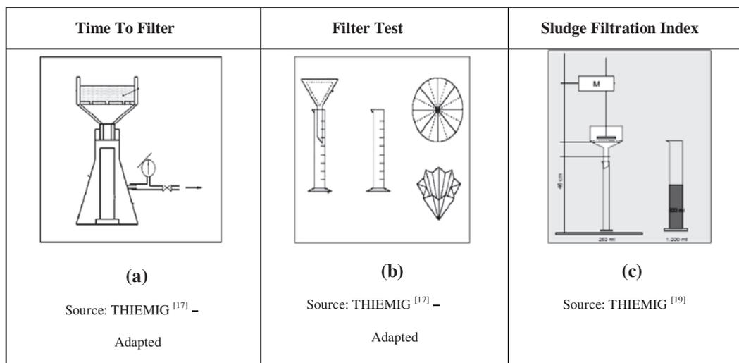
Fig. 1. Assemblies used for sludge filterability tests.
