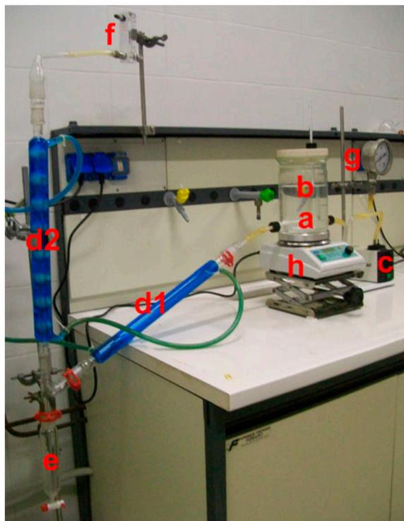
Fig. 2. Laboratory scale unit used for membrane distillation tests.
