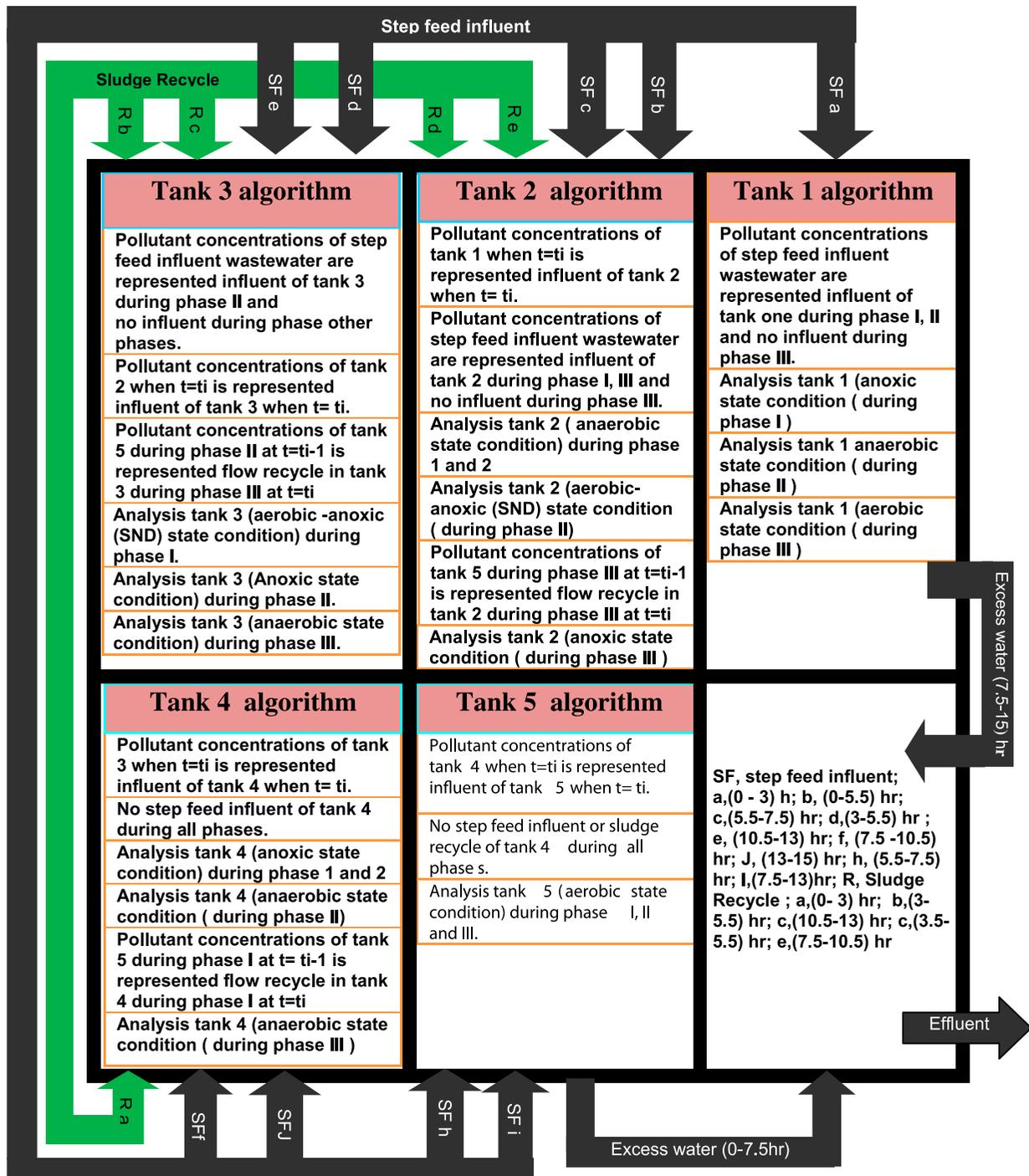
Fig. 4. Layout and algorithms of PITSF-SEU process during a first half cycle.
