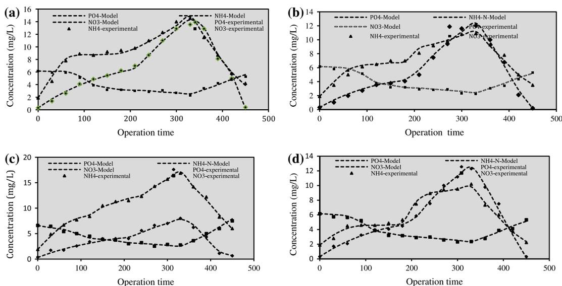
Fig. 6. Experimental data (points) and model simulation (lines) of  $NH_4-N$ , nitrate-N, and  $PO_4-P$  in tank one (a) run 1 (b) run 2 (c) run 3, and (d) run 4.
