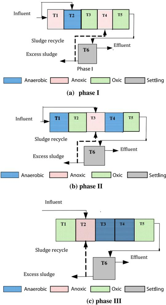
Fig. 5. Diagram of mass balance equation during all phases.
