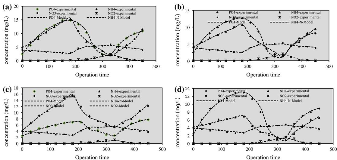
Fig. 7. Experimental data (points) and model simulation (lines) of different soluble components in tank two (a) run 1 (b) run 2 (c) run 3 and (d) run 4.
