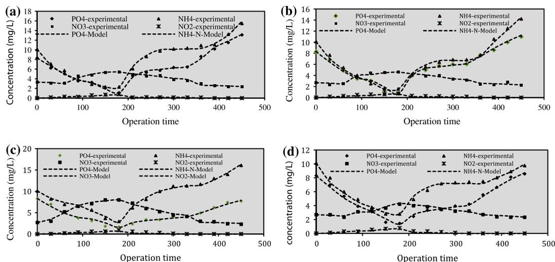
Fig. 8. Experimental data (points) and model simulation (lines) of different soluble components in tank three (a) run 1 (b) run 2 (c) run 3, and (d) run 4.
