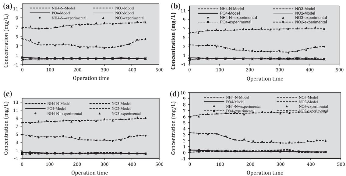
Fig. 10. Experimental data (points) and model simulation (lines) of different soluble components in tank five (a) run 1 (b) run 2 (c) run 3, and (d) run 4.
