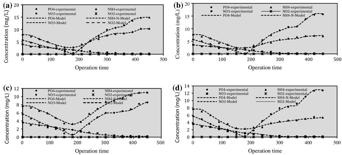
Fig. 9. Experimental data (points) and model simulation (lines) of different soluble components in tank four (a) run 1 (b) run 2 (c) run 3, and (d) run 4.
