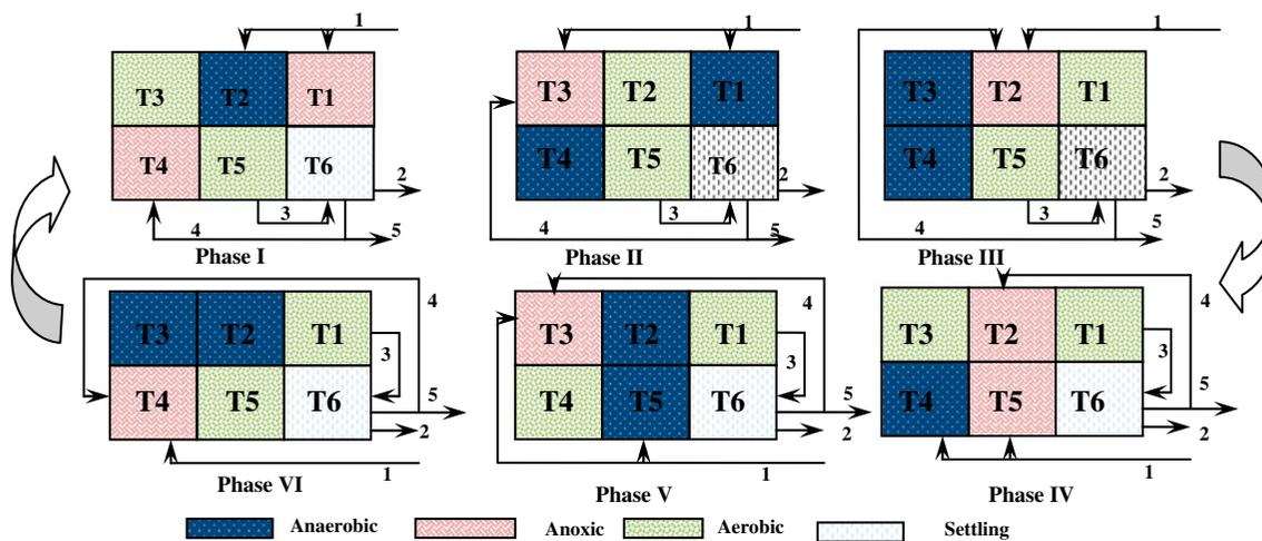
T1–T6, six tanks; 1 - step feed of raw wastewater; 2 - outlet water; 3 - continuous flow of mixed liquor to tank six; 4 - sludge recycle; 5 - excess sludge
