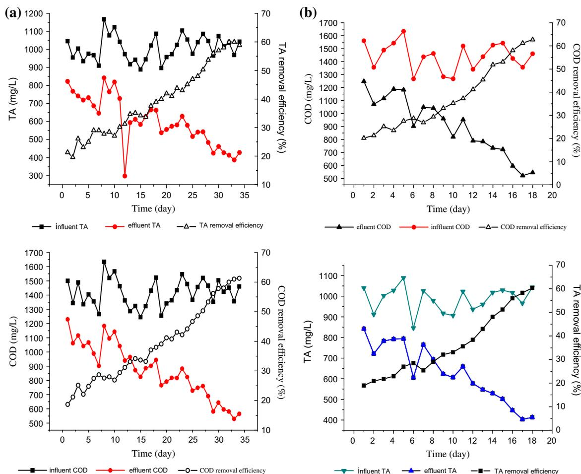
Fig. 5. Performance of (a) R1 and (b) R2 during the start-up period.
