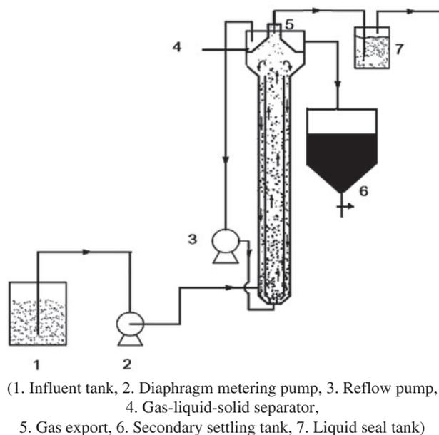
Fig. 1. Schematic diagram of the fluidized bed reactor.
