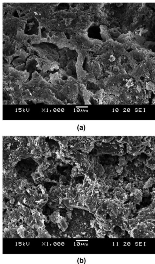
Fig. 2. SEM images of the (a) brick support and (b) porous ceramic support.
