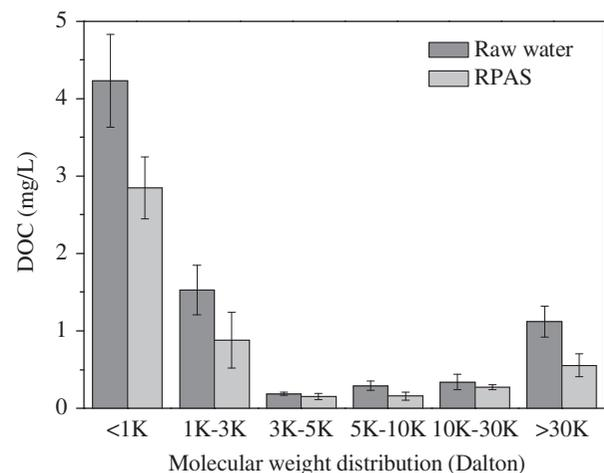
Fig. 9. MW distribution of DOM in raw water and RPAS process effluent.
