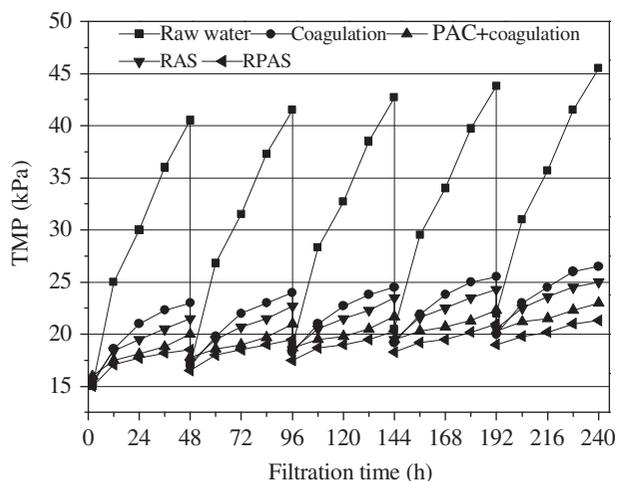
Fig. 5. Comparison of TMP evolution for RASP and other pretreatments during five operating periods (with one operating period of 48 h).
