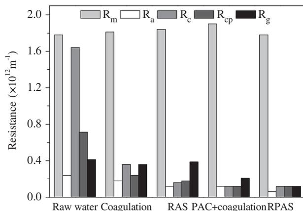
Fig. 3. Effect of RPAS process on the resistance of UF membrane compared to other pretreatments (coagulation, PAC + coagulation and reuse of alum sludge).
