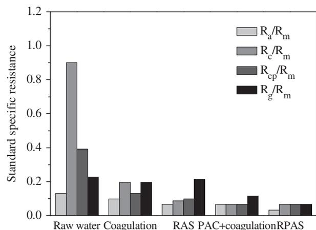
Fig. 4. Standard specific resistance of UF membrane for different pretreatments (coagulation, PAC + coagulation, reuse of alum sludge and reuse of PAC and alum sludge).
