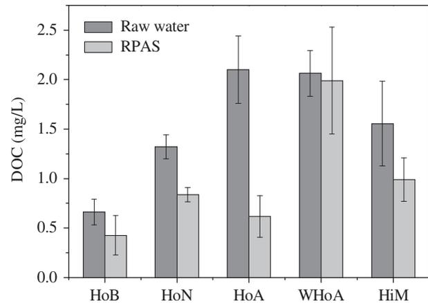
Fig. 8. Fractionation of DOM in raw water and RPAS process effluent.
