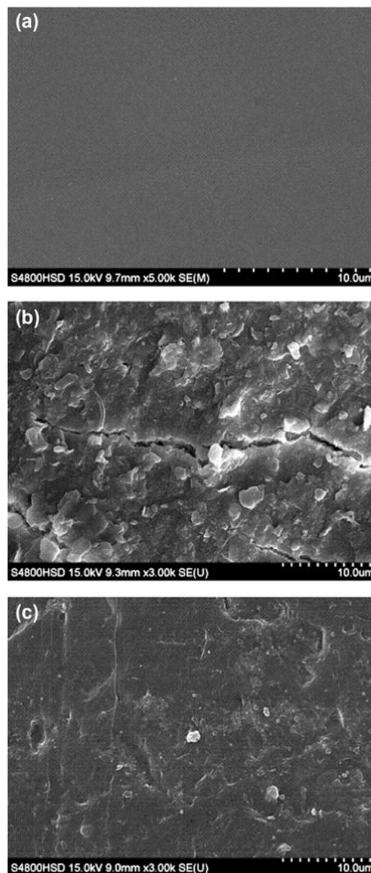
Fig. 6. SEM images of clean membranes surface (a), as well as fouling layer on the membrane surface after filtrating raw water (b) and RPAS effluent (c).
