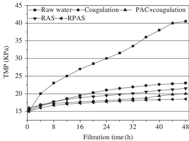
Fig. 2. TMP evolution of RPAS coupled with UF compared with three other different pretreatments (coagulation, PAC + coagulation and reuse of alum sludge).
