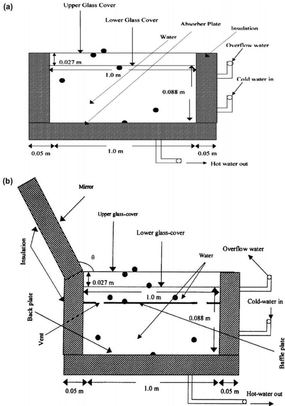
Fig. 1. (a) Shallow solar pond with double glass cover, adapted from: Aboul-Enein et al. [42]. (b) Shallow solar pond with baffle plate, adapted from El-Sebaï [75].
