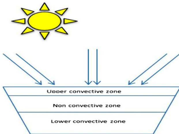
Fig. 2. SGSP, adapted from Hull [65].
