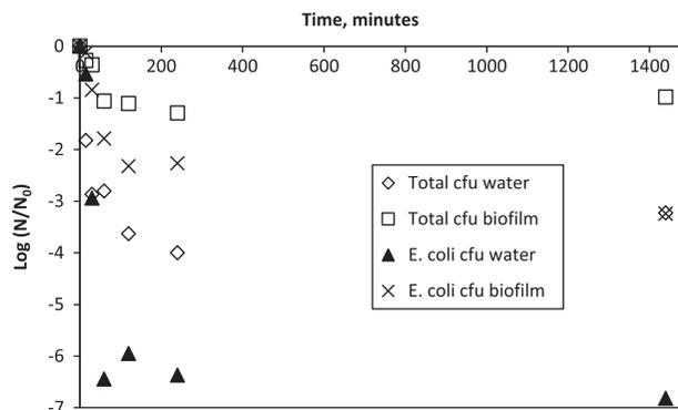
Fig. 3. Log reduction of cultivable microorganisms (as HPC) and cultivable *E. coli* in water and biofilm after chlorine inactivation for 24 h. The data represent the average from three separate runs. The detection limits for both methods were estimated as 6 log.
