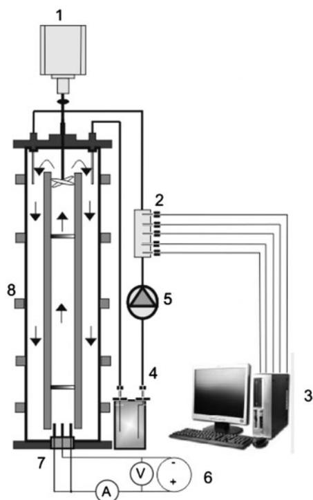
Fig. 1. Schematic overview of the electrochemical disinfection unit. (1) electric motor; (2) sensor cell; (3) data logger connected to PC; (4) extra water sample supply (1 L); (5) peristaltic pump; (6) direct current source; (7)  $\text{TiO}_{2-x}$  ceramic electrodes; and (8) Propella™ reactor with 20 biofilm sampling devices.
