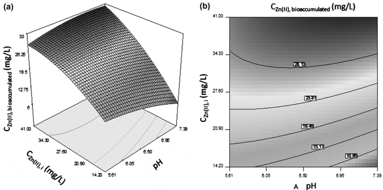
Fig. 6. (a) Response surface plot described by the model  $Y_2$ , which represents the effect of pH and initial Zn(II) ion concentration and their mutual effects on Zn(II) bioaccumulation and (b) response surface contour plot of Zn(II) bioaccumulation showing interactive effect of pH and initial Zn(II) ion concentration.
