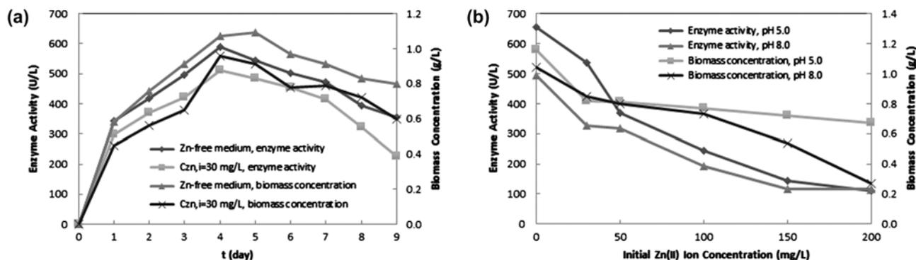
Fig. 1. (a) Growth and simultaneous lipase production curves of *R. delemar* at pH 5.0 and 25°C in the medium containing 30 mg/L initial Zn(II) ion concentration and in the Zn(II)-free fermentation medium and (b) Change of enzyme activity and biomass concentration with initial Zn(II) ion concentration at pH 5.0 and 8.0 and at 35°C.
