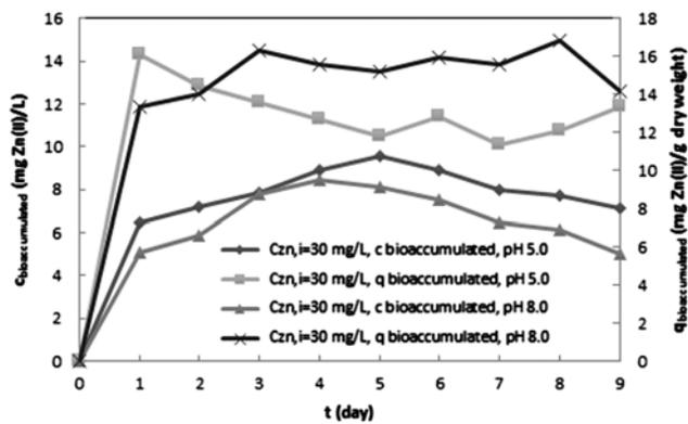
Fig. 2. Time course of bioaccumulated Zn(II) ion concentration (mg/L) and bioaccumulated Zn(II) ion quantities per unit mass of biomass on dry weight basis (mg Zn(II)/g dry weight) at pH 5.0 and 8.0 and at 25°C.
