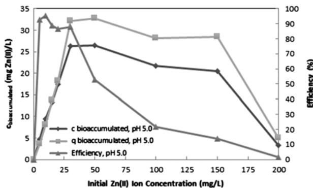
Fig. 3. Change of bioaccumulated Zn(II) ion concentration (mg/L), bioaccumulated Zn(II) ion quantities per unit mass of biomass on dry weight basis (mg Zn(II)/g dry weight), and bioaccumulation efficiency at pH 5.0 and at 35°C.
