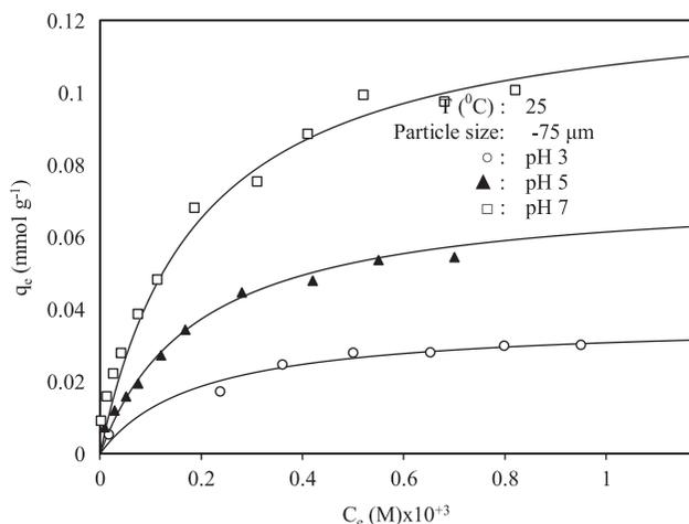
Fig. 7. The effect of suspension pH on adsorption capacity of hazelnut shell.
