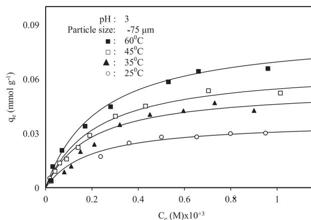
Fig. 8. The effect of temperature on adsorption capacity of hazelnut shell.
