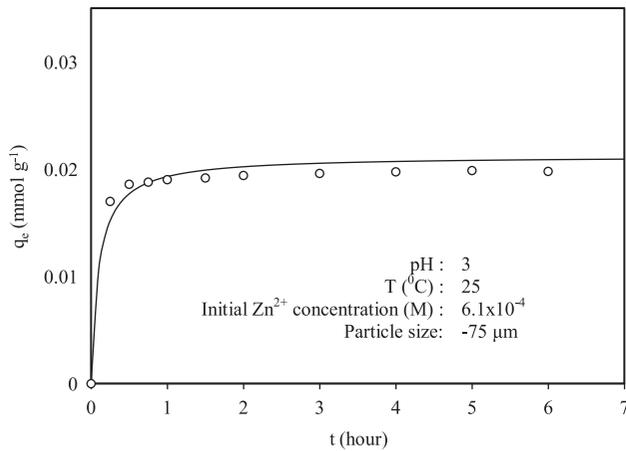
Fig. 5. Adsorption capacity as a function of incubation time of hazelnut shell.
