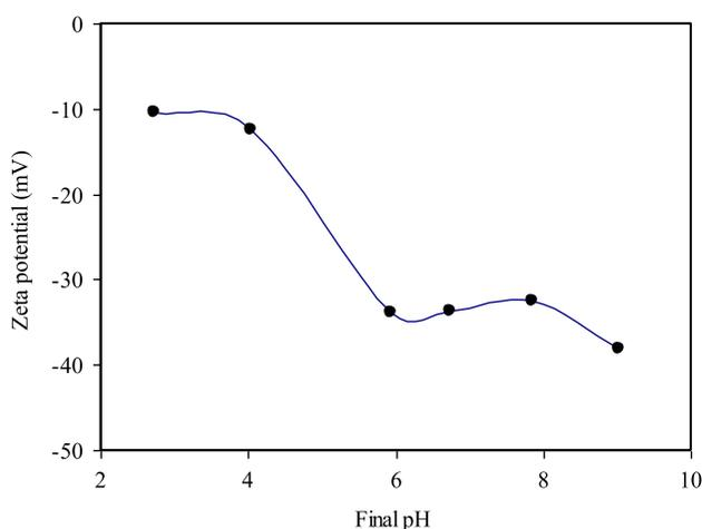
Fig. 3. The variation of zeta potential with equilibrium pH of hazelnut shell suspensions at 25 °C, 75 µm particle size.
