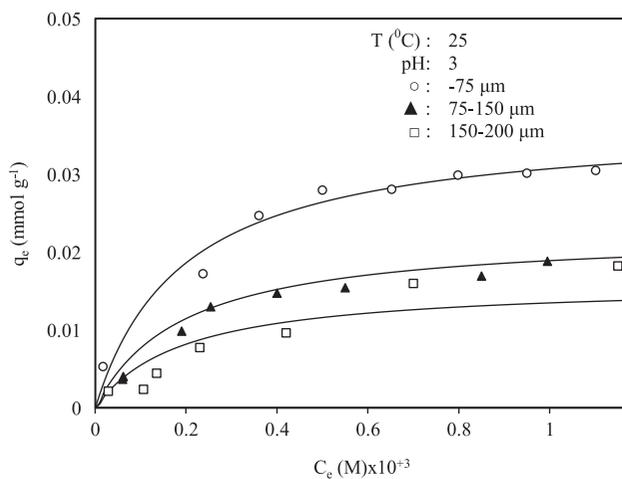
Fig. 6. The effect of particle size on adsorption capacity of hazelnut shell.
