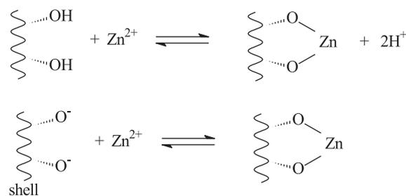
Fig. 4. Possible mechanisms of ion exchange.
