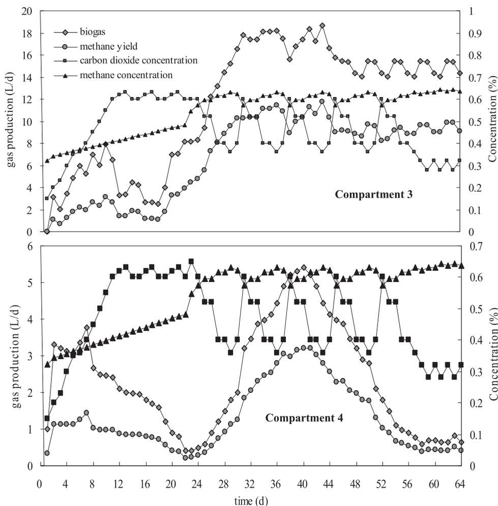
Fig. 4. Variation of biogas yields and gas concentration in the methane production process.
