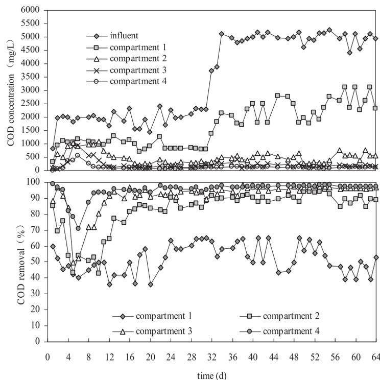
Fig. 6. COD concentration and removal contribution of each compartment in ABR.
