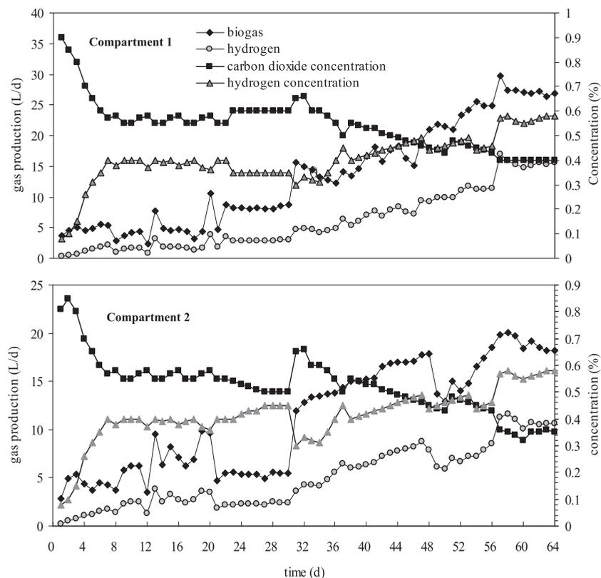
Fig. 2. Variation of gas yields and hydrogen concentration in the hydrogen production process.
