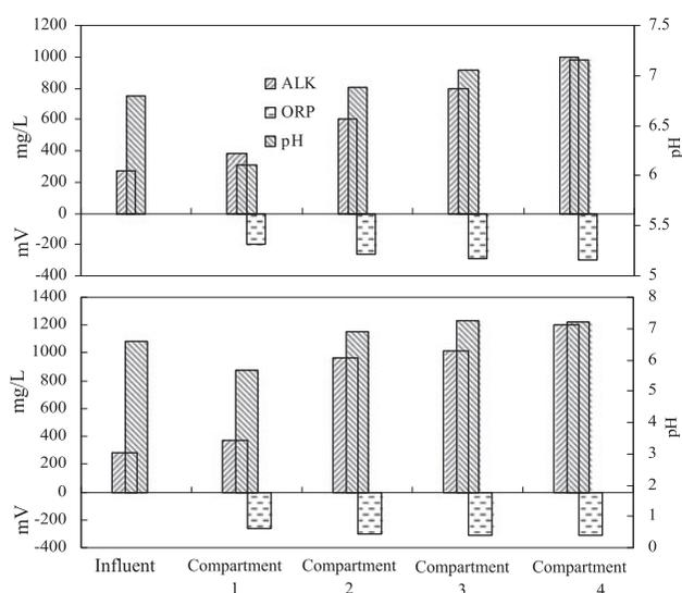
Fig. 7. The variation of pH, ALK, and ORP in the ABR for energy recovery.
