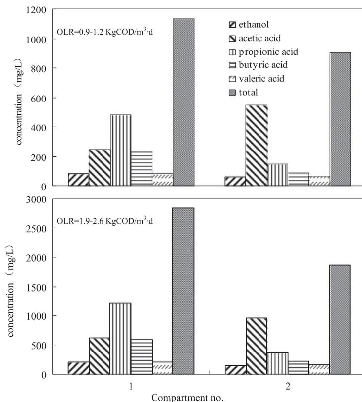
Fig. 3. VFAs and ethanol in the hydrogen production compartments with OLR.
