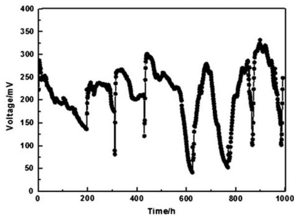
Fig. 4. Voltage generation by double-chambered MFC.
