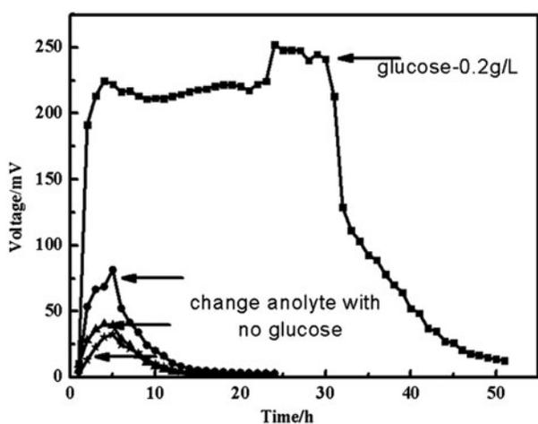
Fig. 3. Voltage generation by MFC 1-1 during start-up. Note: ■: with glucose; ●: the first time anolyte replaced without glucose; ▲: the second time anolyte replaced without glucose; ▼: the third time anolyte replaced without glucose.
