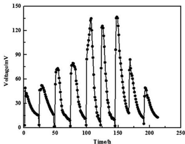
Fig. 2. Voltage generation by MFC 1-2 during start-up.
