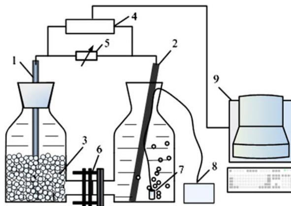
Fig. 1. Schematic diagram of double-chambered MFC. Note: 1: anode; 2: cathode; 3: granule graphite; 4: data recorder; 5: resistance box; 6: PEM; 7: aerator; 8: oxygen pump; 9: computer.
