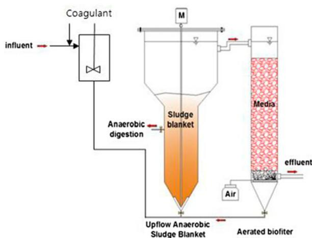
Fig. 1. Schematic diagram of lab-scale UASB-ABF system.
