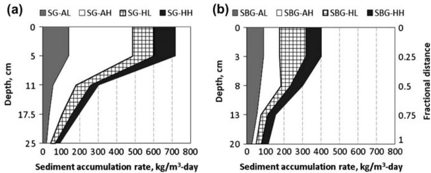
Fig. 4. Sediment accumulation with respect to the depth in the (a) infiltration and (b) retention column.
