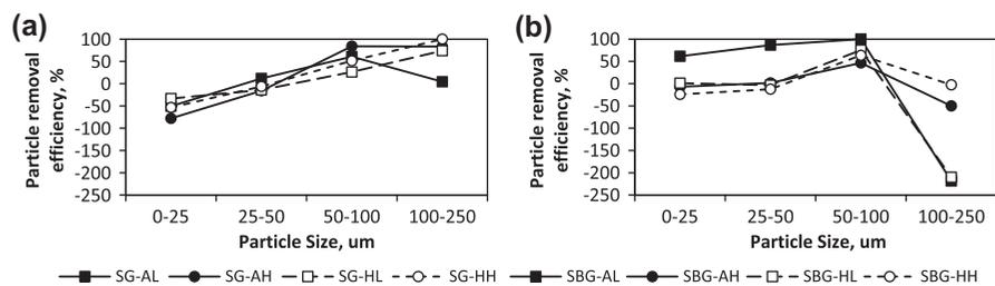
Fig. 3. Particle retention efficiency between the inflow and final outflow water samples in (a) infiltration and (b) retention columns.
