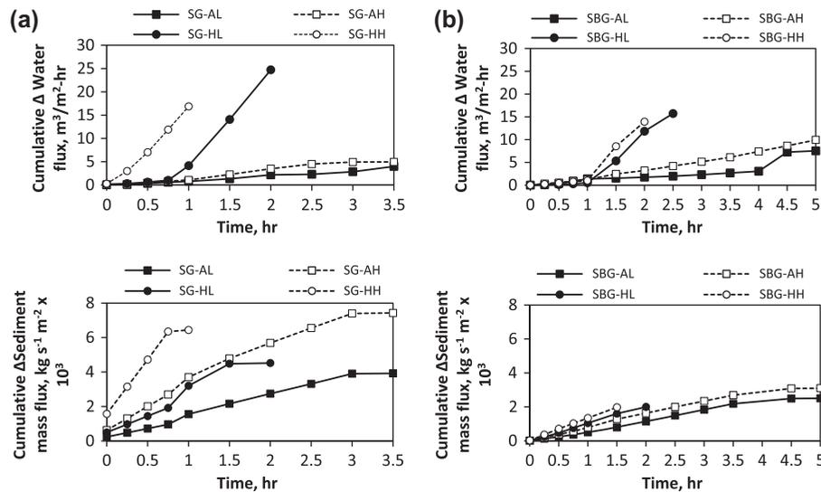
Fig. 2. Cumulative change in flux and cumulative change in mass flux of the (a) infiltration and (b) retention columns.
