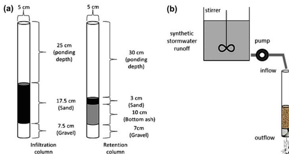
Fig. 1. (a) Infiltration and retention column and (b) experimental setup schematic.
