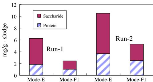
Fig. 4. ECP contents of the sludges (Mode-F1: clogging period).
