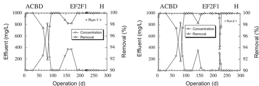
Fig. 5. Profiles of effluent concentration and removal of phenol.
