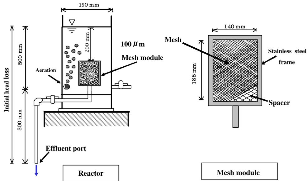
Fig. 1. Schematic diagram of the mesh filtration bio-reactor.
