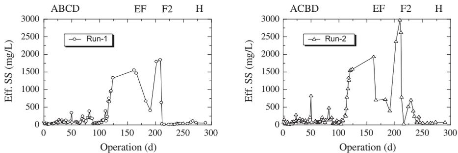
Fig. 3. Profiles of SS of the effluents.
