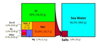
Fig. 7. Typical chemical composition of seawater. Note: Numbers in brackets represent the mass of each constituent for 1 kg of seawater.
