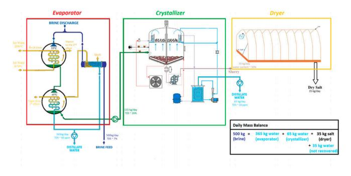
Fig. 6. Process flow diagram of the SOL-BRINE system. Note: The figures represent the daily mass balance of the system.
