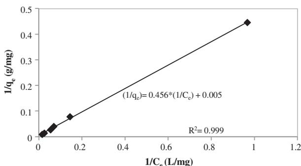
Fig. 7. Linear transform of Langmuir isotherm.
