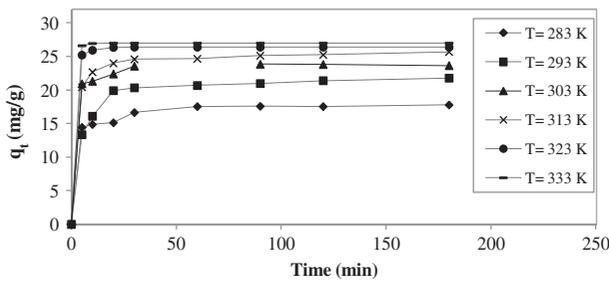
Fig. 6. Effect of temperature on the amount of MB adsorbed on Alfa grass ( $C_0=100\text{ mg/L}$ ;  $\text{pH}=12$ ;  $N=500\text{ rpm}$ ).
