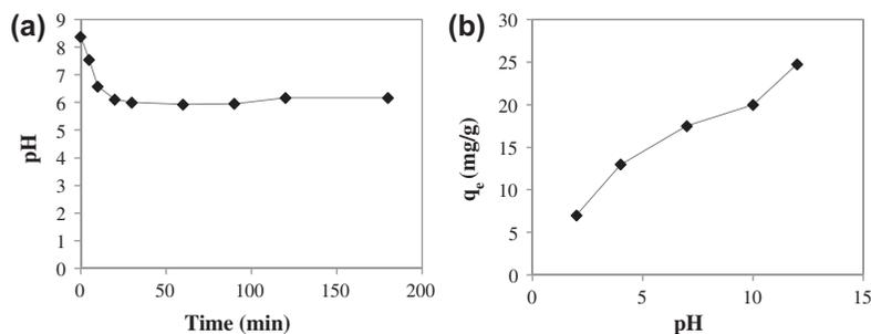
Fig. 4. (a) Evolution of pH solution and (b) evolution of equilibrium adsorption capacity with pH ( $T=293$  K;  $C_0=100$  mg/L;  $N=500$  rpm;  $W=400$  mg).
