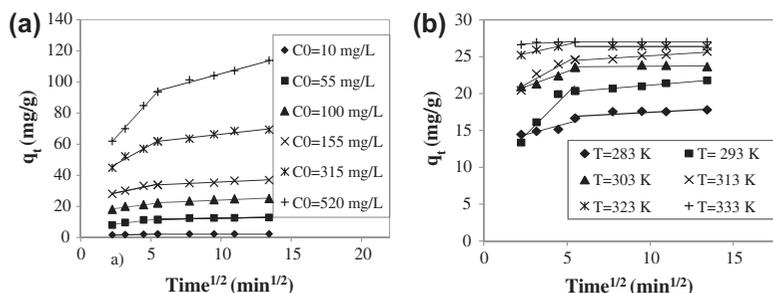
Fig. 9. Intraparticle diffusion plots for MB adsorption on Alfa grass.
