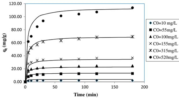
Fig. 8. Experimental data and simulated kinetics for various initial MB concentrations.
