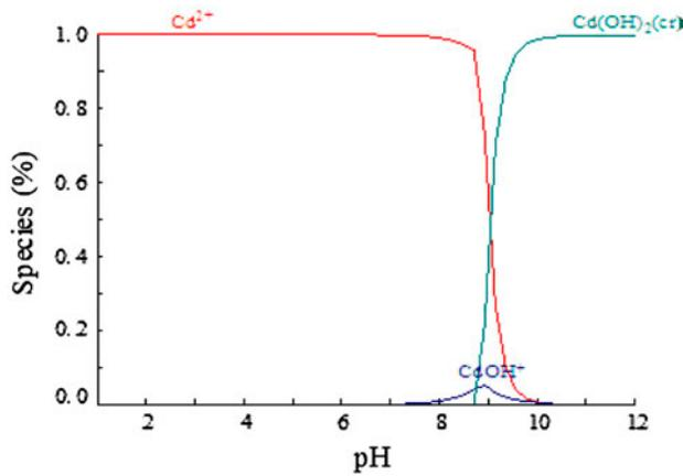
Fig. 2. Species fraction diagrams vs. pH (10 mg/L cadmium nitrate).
