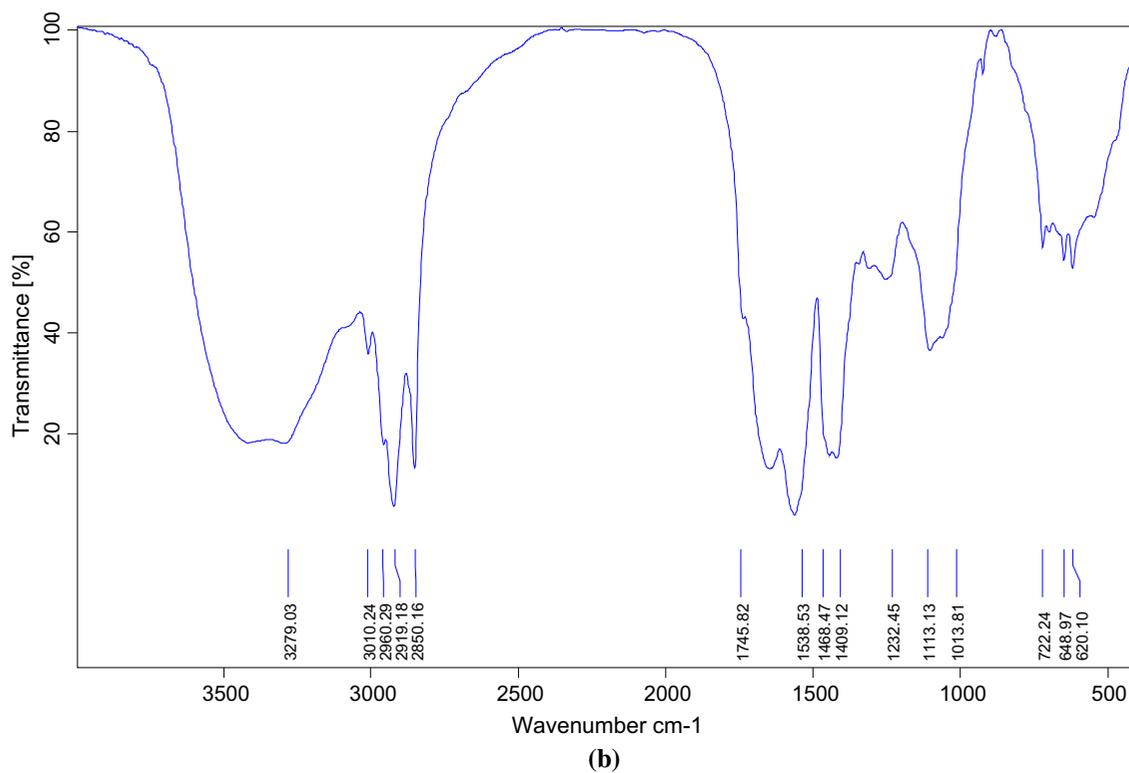
Fig. 7. FTIR spectra of Cd-free *A. protothormiae* (a) and Cd (II)-loaded *A. protothormiae* biomass (b).
