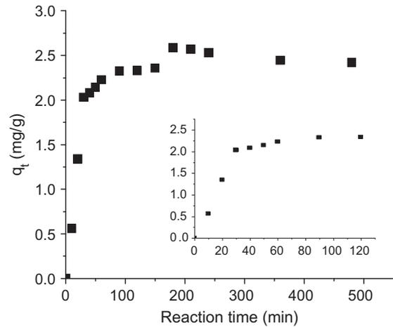
Fig. 4. Kinetics of Cd (II) adsorption by *A. protophormiae* biomass (pH 7, reaction temperature: 25 °C, Cd (II) initial concentration: 10 mg/L, adsorbent concentration: 5 kg/m<sup>3</sup>). The inset shows the  $q_t$  vs. reaction time at <120 min.
