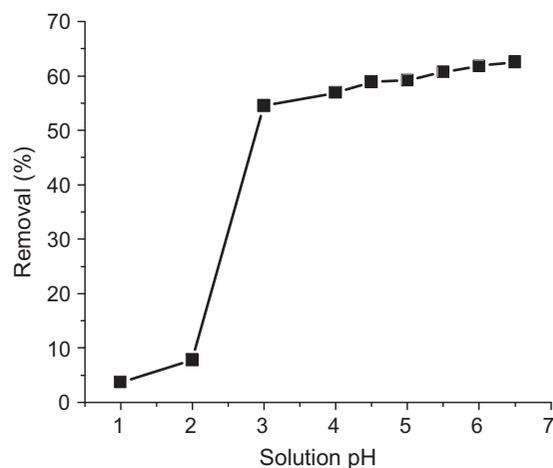
Fig. 1. Cd (II) adsorption by *A. protophormiae* biomass as a function of pH (Cd (II) initial concentration: 10 mg/L, adsorbent concentration: 5 g/L, reaction temperature: 25°C, contact time 2 h).
