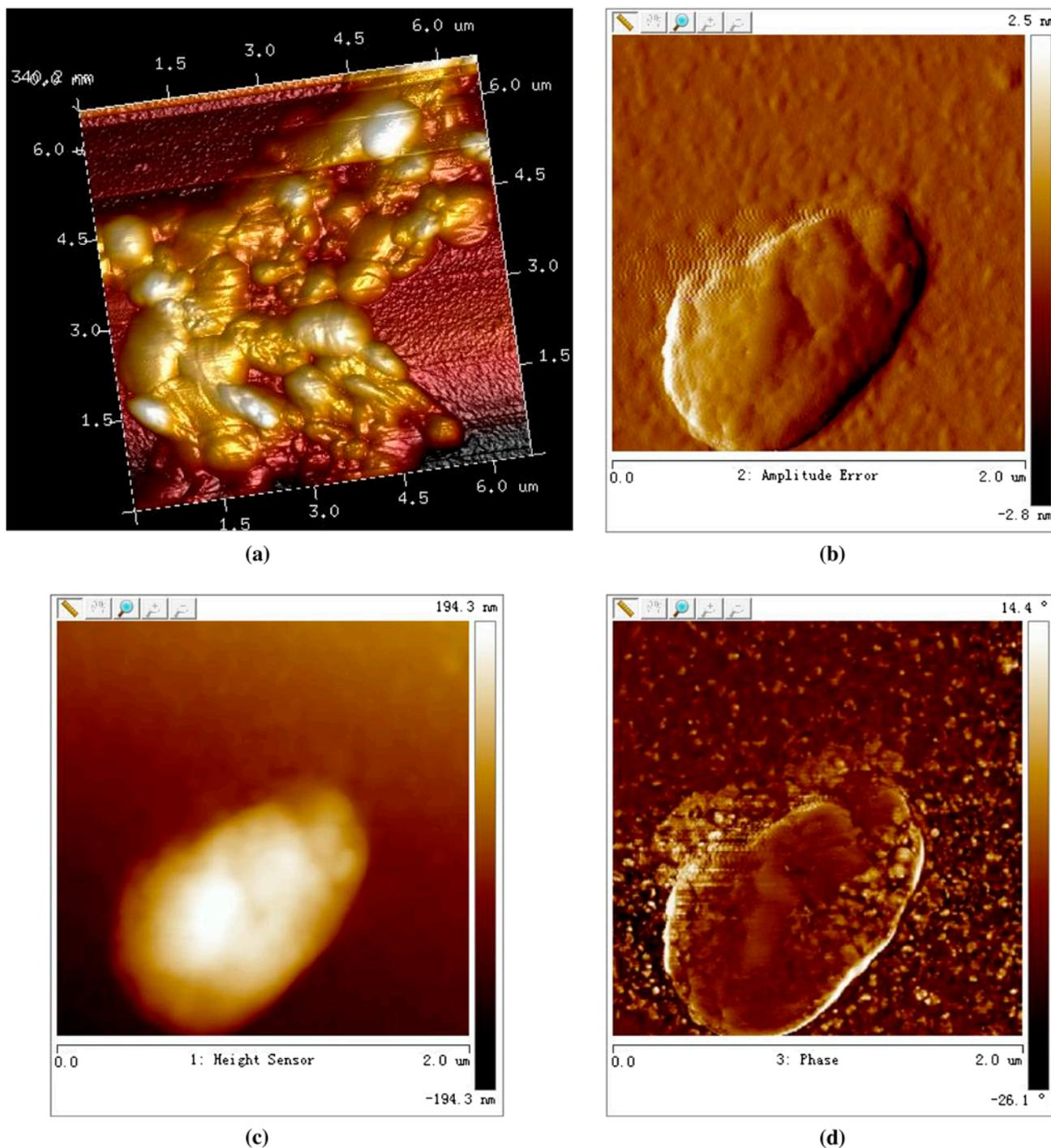
Fig. 10. AFM microscopic images of bacterial cells loaded with Cd (II) (a: three-dimensional image, b: amplitude image; c: height image; d: phase image).
