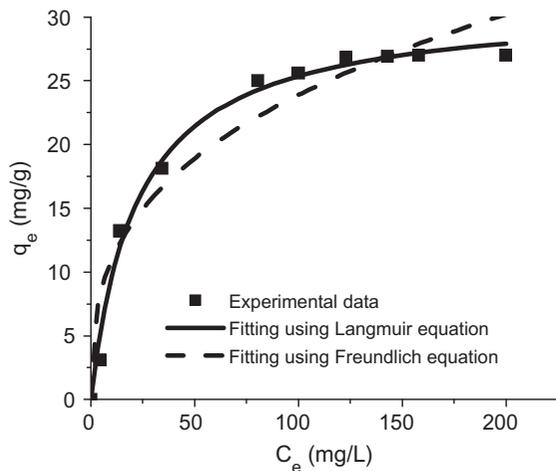
Fig. 6. Cd (II) adsorption isotherm on *A. protothormiae* biomass with the results fitted to the Langmuir and Freundlich isotherms (Contact time 8 h, pH 7, reaction temperature 25°C, adsorbent concentration 5 kg/m<sup>3</sup>).
