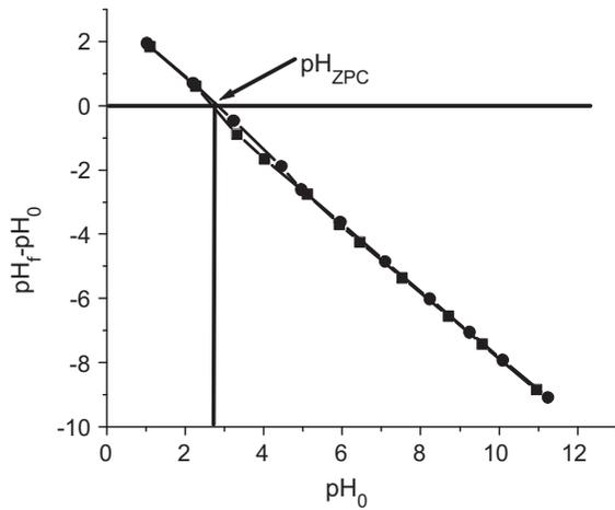
Fig. 3. Net surface charge of *A. protophormiae* biomass as a function of initial solution pH.
