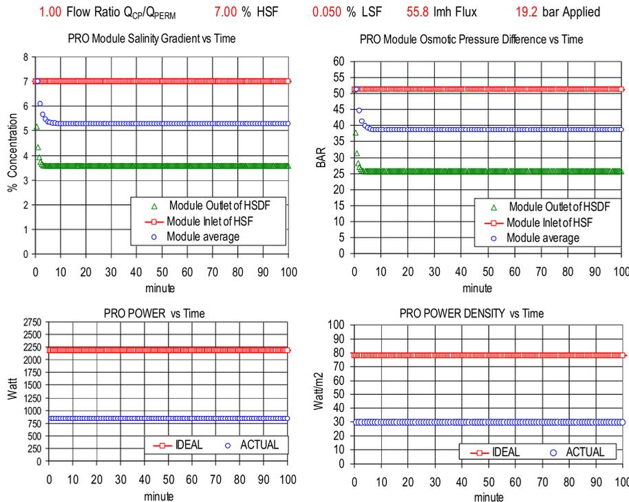
Fig. 7. CC-PRO performance characteristics of a single module CC-PRO unit with the salinity gradient system 0.05–7.0% under the conditions specified in Table 2.
