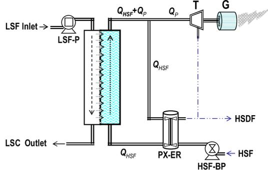
Fig. 1. Illustration of a single module conventional PRO power generation system.
