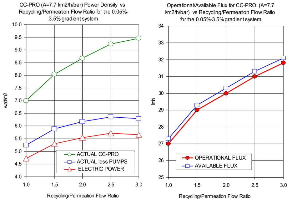
Fig. 6. Power output of the CC-PRO unit with the salinity gradient system 0.05–3.5% under the conditions specified in Table 1 except for recycling/permeation flow ratio changes in the range 1.0–3.0 with actual flux selection of 0.3lmh below the available flux.
