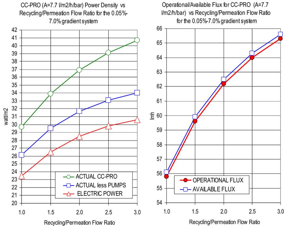
Fig. 8. Power output of the CC-PRO unit with the salinity gradient system 0.05–7.0% under the conditions specified in Table 2 except for recycling/permeation flow ratio changes in the range 1.0–3.0 with actual flux selection of 0.3lmh below the available flux.
