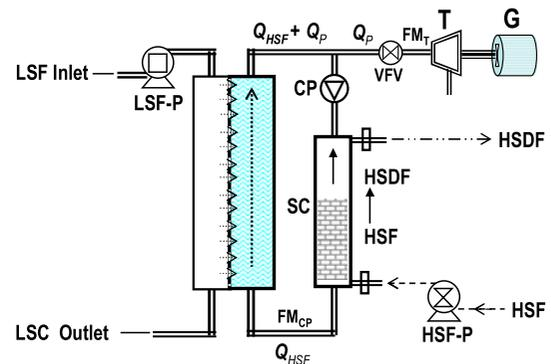
Fig. 2B. A single module batch CC-PRO apparatus with power generation stopped to enable HSDf replacement by fresh HSF at near atmospheric pressure by means of the HSF-P pump.
