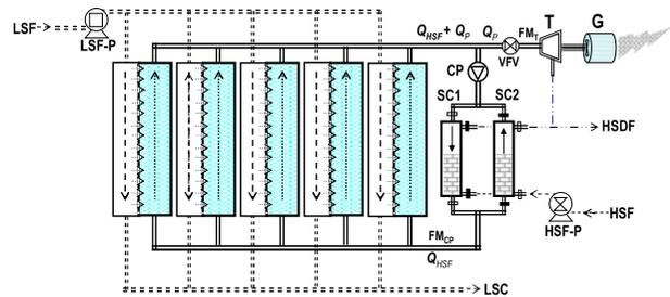
Fig. 4. A five modules CC-PRO apparatus for continuous power generation by a consecutive sequential batch process with two alternating SCs without need for ER.
