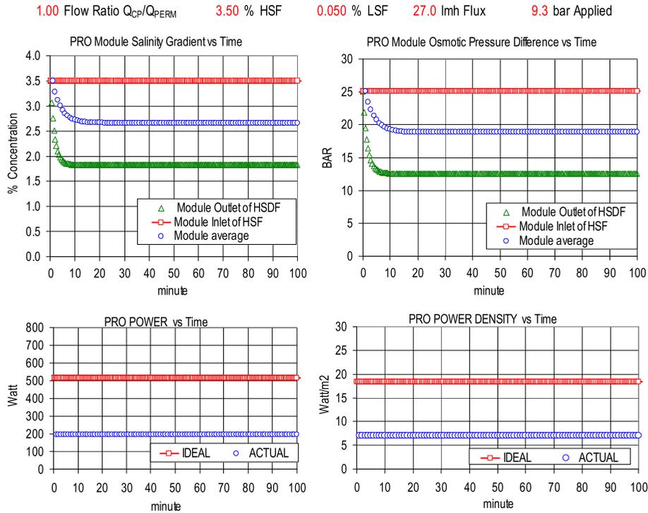
Fig. 5. CC-PRO performance characteristics of a single module CC-PRO unit with the salinity gradient system 0.05–3.5% under the conditions specified in Table 1.
