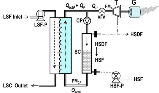
Fig. 2A. A single module batch CC-PRO apparatus in operation performing power generation in CC through a SC without need of energy recovery.
