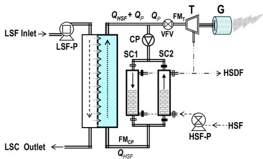
Fig. 3. A single module CC-PRO apparatus for continuous power generation by a consecutive sequential batch process with two alternating SCs without need for energy recovery.
