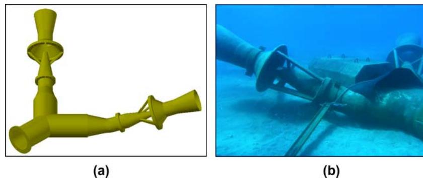
Fig. 3. Diffuser system with Y bifurcation and 90° aperture from where the two branches decreasing from 600/400 mm Ø lead off, where the conventional diffuser nozzles with reduced outlets of 130 mm Ø are inserted, with the venturi effect suction unit incorporating replaceable and interchangeable attachment systems: (a) image of the design, (b) photo of the device in place.
