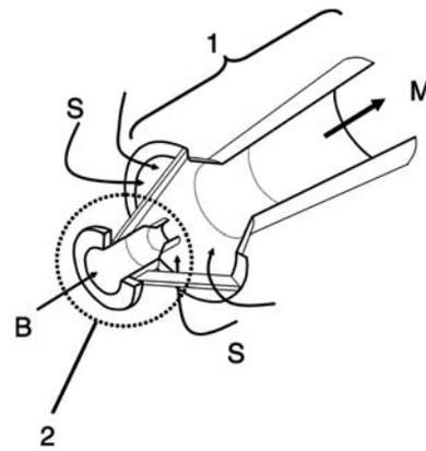
Fig. 1. Venturi eductor: Diffuser system comprising a conventional diffuser nozzle, or reducer nozzle (2), where the exit velocity of the brine discharge increases (B) after attachment of a venturi effect trumpet-shaped structure (1) through which ambient water is suctioned (S); the mixture emerges through the exit (M).
