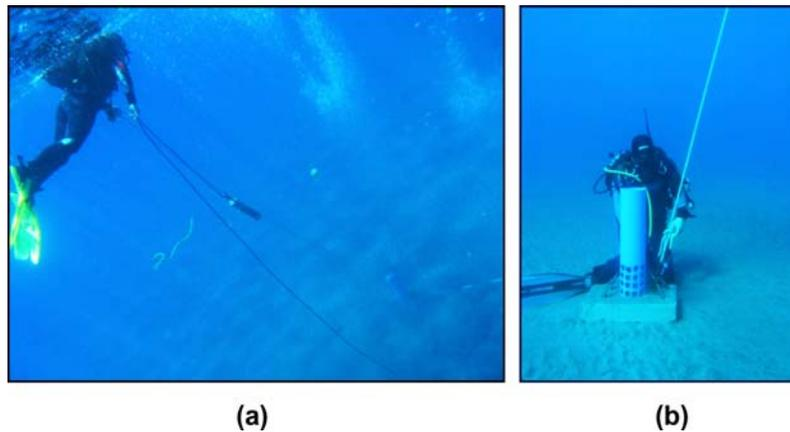
Photo 2. (a) Profile of the start of the far field, showing the diver holding the marker buoy rope tight and lowering a YSI-6600-V2 multiparameter sensor to the sea bottom, where the other sensor is anchored and taking continuous measurements; (b) Perforated cylindrical PVC tube attached to a mooring block (weighing approximately 50 kg fully loaded) to anchor a second YSI-6600-V2 multiparameter sensor in a vertical position.
