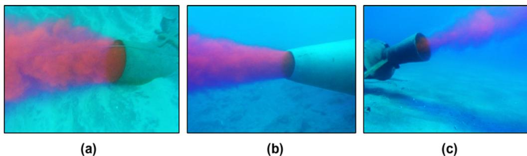
Photo 1. Addition of rhodamine during near-field sampling: (a) with no diffuser system; (b) with the reducer nozzle; and (c) with the suction unit.
