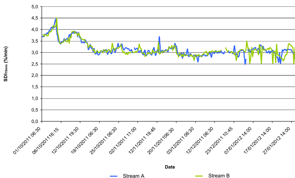
Fig. 6. Pre-treated water SDI 15min during the first months of the plant operation.
