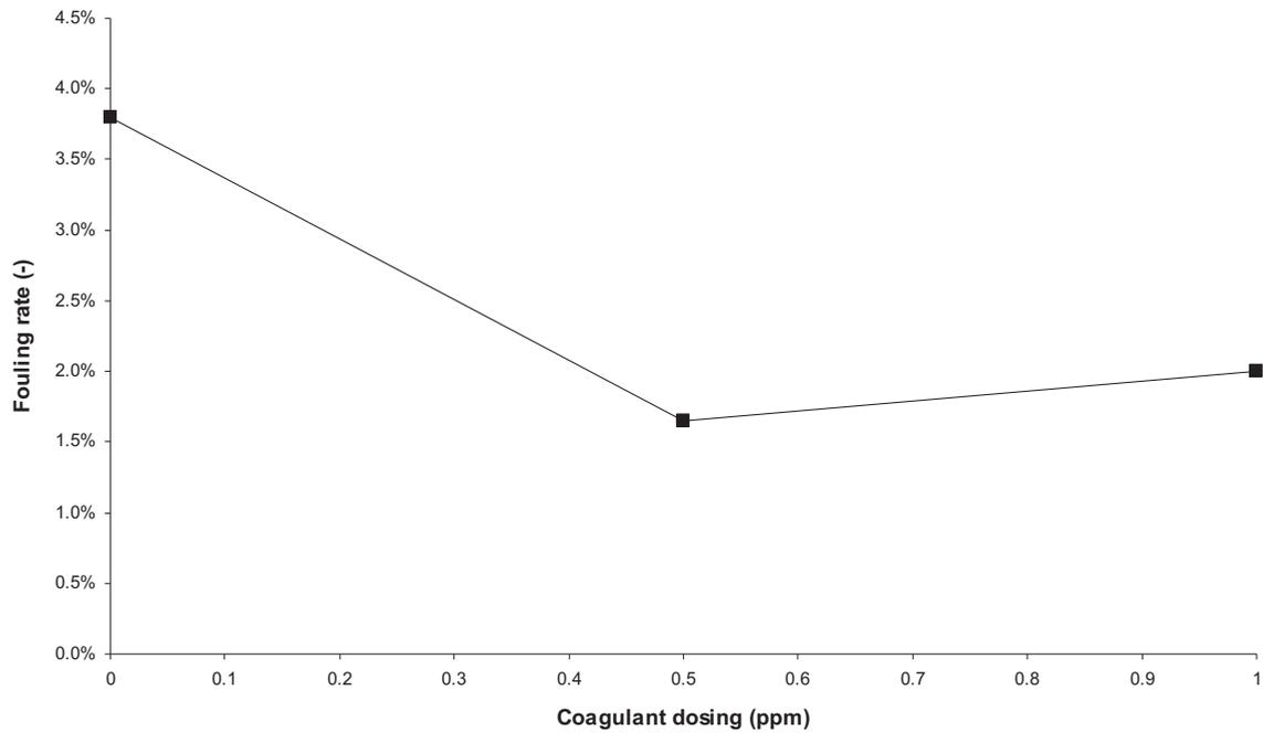
Fig. 10. Fouling rate as a function of coagulant dose (Twente canal water, 751/m<sup>2</sup>-h).
