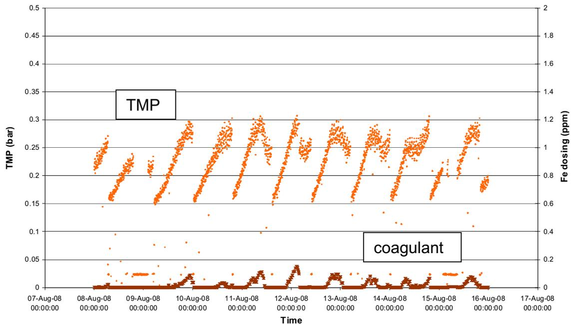
Fig. 11. Dynamic coagulant dosing in practice (seawater: flux is 1001/m<sup>2</sup>-h with an internal recirculation of 15%).
