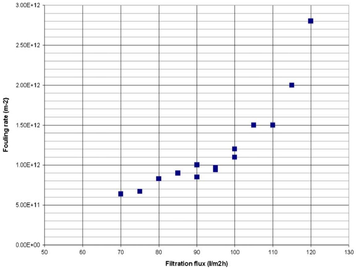
Fig. 8. Fouling rate as a function of filtration flux (Twente canal water (45–60 NTU), 15% circulation, no coagulant dosing).
