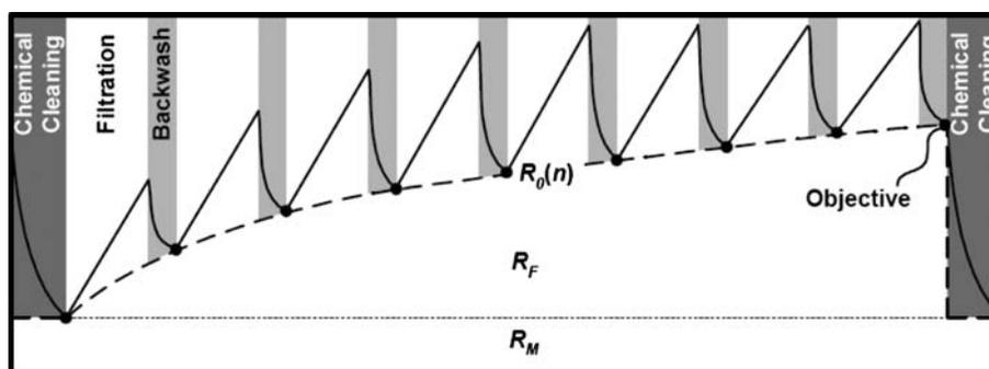
Fig. 6. Series of subsequent filtrations and backwashes between two chemical cleaning phases. The dashed line illustrates the development of the (ideal) resistance trajectory.
