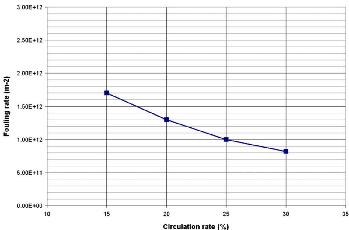
Fig. 9. Fouling rate as a function of recirculation rate (Twente canal water, during algae bloom 45–60 NTU, 1001/m<sup>2</sup>-h, no coagulant).
