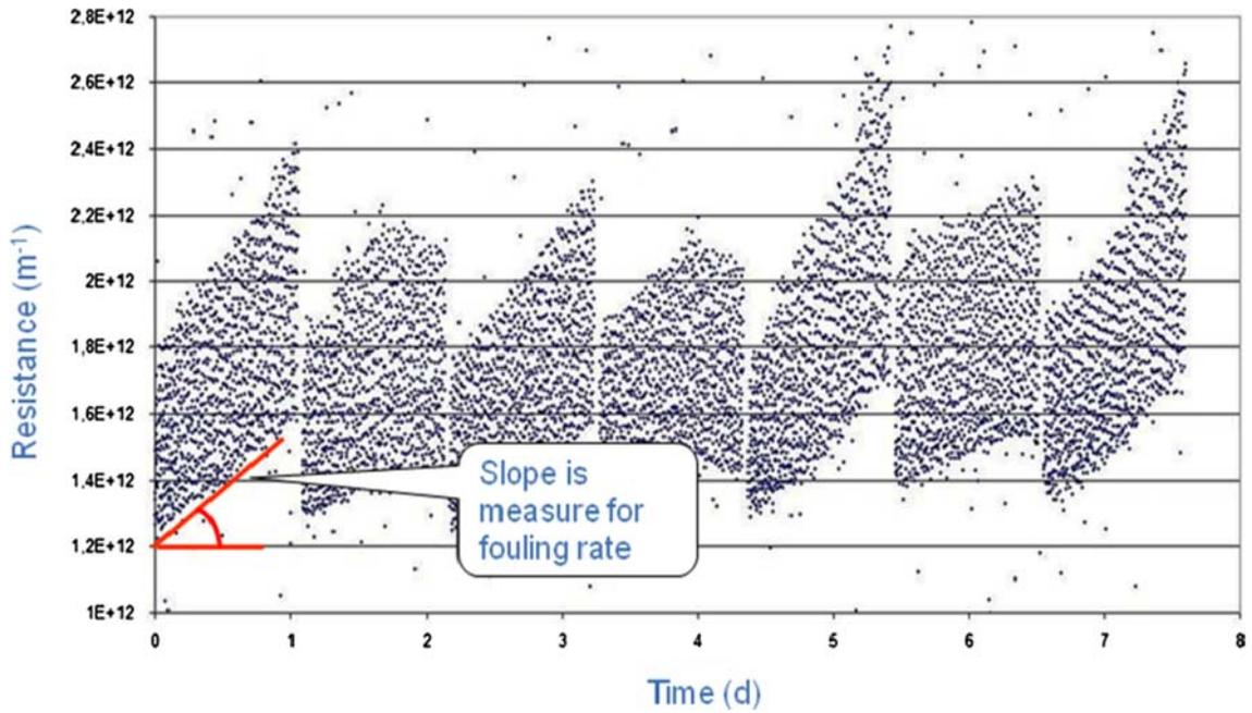
Fig. 7. Overall filtration resistance as a function of filtration time (Twente canal water (45–60 NTU), 15% circulation, no coagulant dosing).
