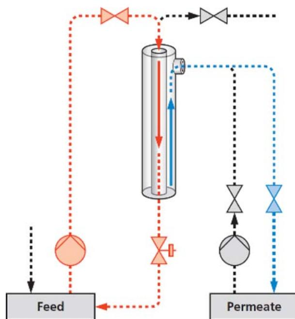
Fig. 3. AquaFlex™ processing: semi-dead-end with a small circulation flow.
