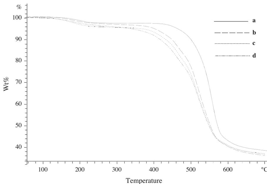
Fig. 9. TGA thermograms of: (a) PES and (b)–(d) PES + poly(CBMA-TMC) blends; CBMA = 2%, TMC = 0.01, 0.1 and 0.2% in b, c, and d, respectively.
