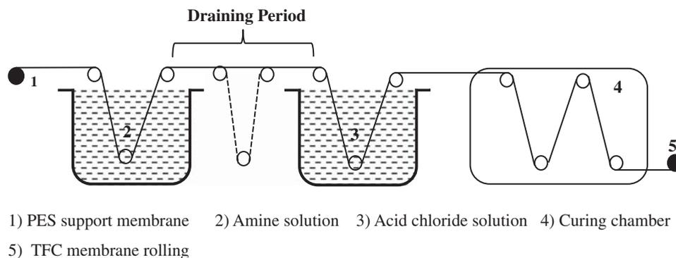
Fig. 1. Schematic diagram for the preparation of polyamide skin layer on the PES support membrane.
