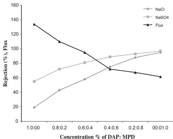
Fig. 5. Variation of the membrane performance with DAP-MPD composition in polyamide skin. TMC concentration = 0.1%, feed concentration = 2,500 ppm, pressure = 10 kg/cm<sup>2</sup>.
