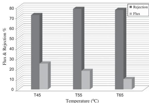
Fig. 7. Variation of membrane performance with the curing temperature of a polyamide skin. CBMA = 2%, TMC = 0.2%; feed = NaCl (2,500 ppm), pressure = 10 kg/cm<sup>2</sup>.
