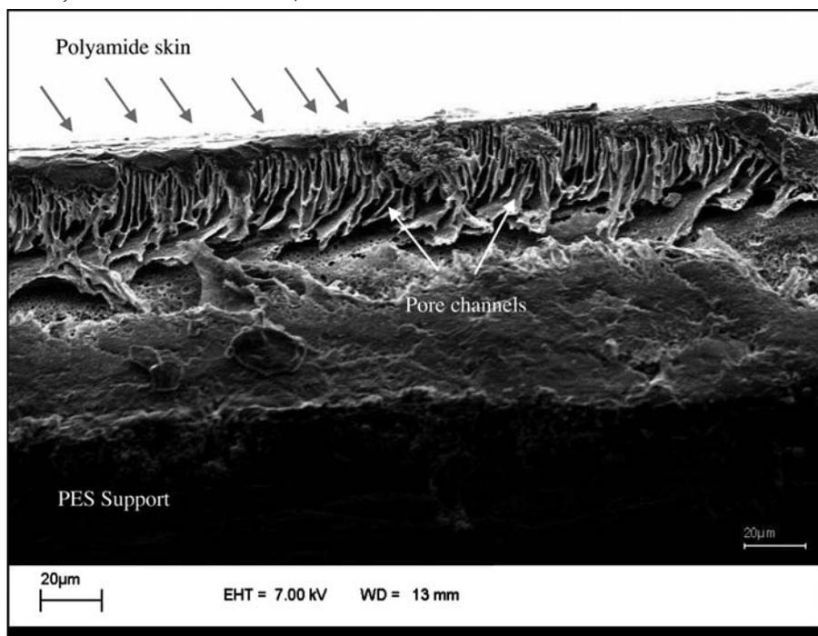
Fig. 8. SEM cross-section microphotograph of a poly(CBMA-TMC) composite membrane.
