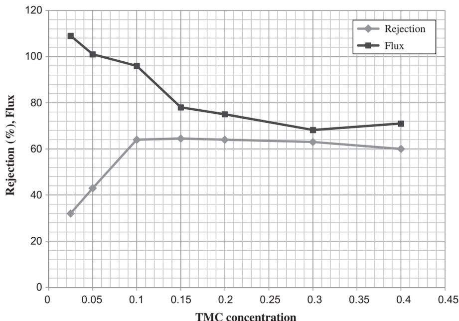
Fig. 6. Variation of membrane performance with acid chloride (TMC) concentration, amine (MPD:PIP=0.5:0.5%), feed = NaCl (2,500 ppm), pressure = 10 kg/cm<sup>2</sup>.
