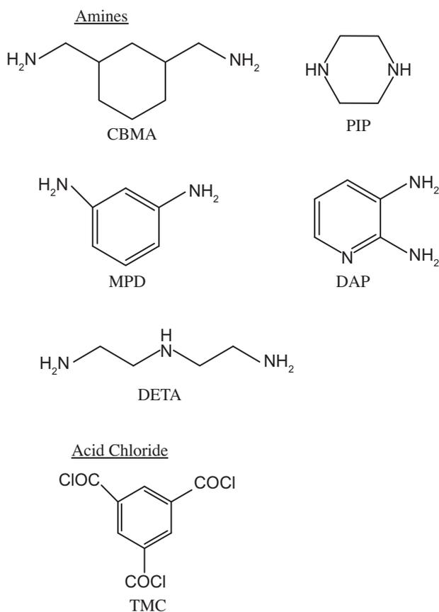
Fig. 2. Chemical structures of monomers.
