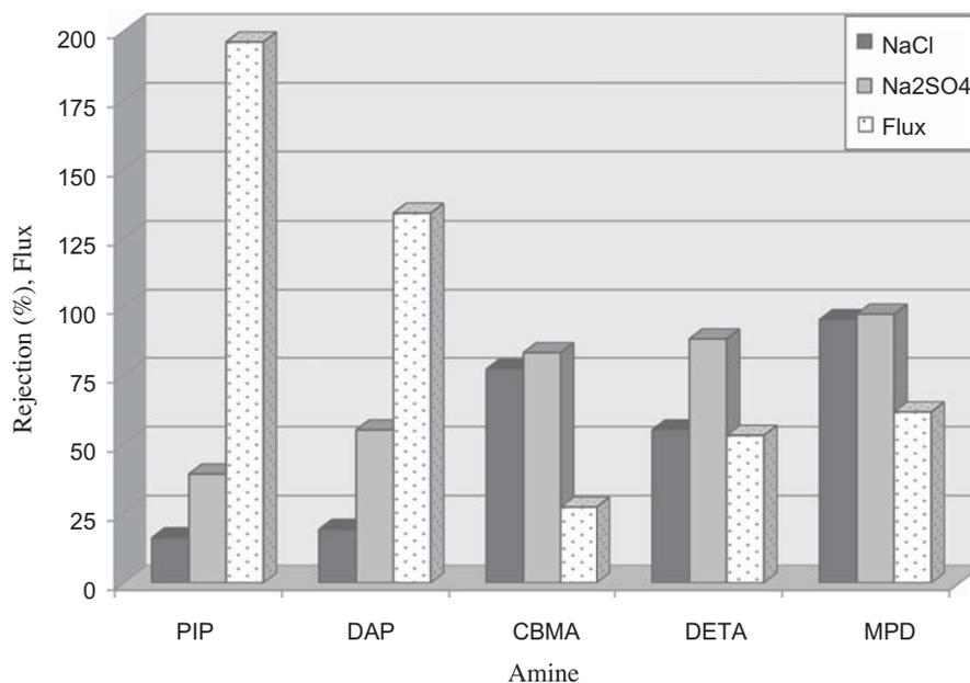
Fig. 4. Dependence of the membrane performance on the chemical nature of polyamide skin TMC concentration = 0.1%, feed concentration = 2,500 ppm, pressure = 10 kg/cm<sup>2</sup>.
