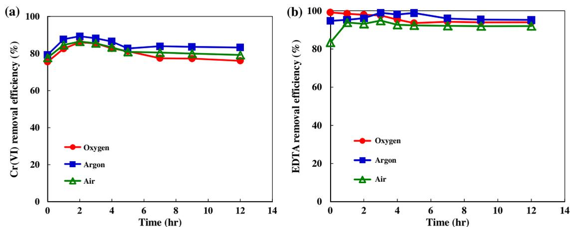
Fig. 7. A comparison of the removal efficiencies for the (a) reduction of Cr(VI) and (b) oxidation of EDTA with  $\text{TiO}_2$  under UV irradiation for different oxygen contents, aerated by argon, air and oxygen, respectively (both Cr(VI) and EDTA=0.001 M, pH=3.0, HRT=4.0 h).
