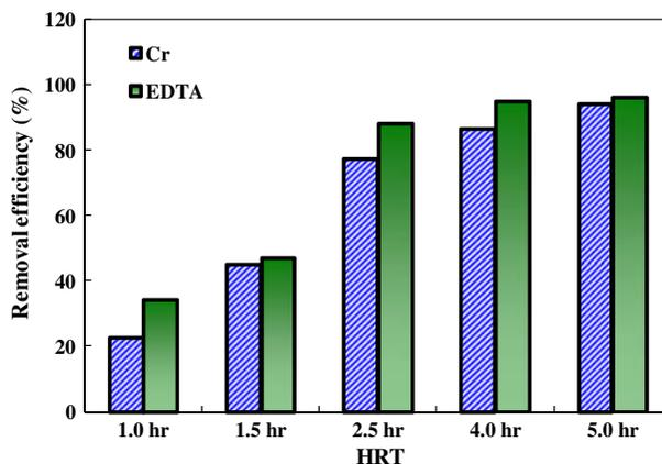
Fig. 5. A comparison of the removals of Cr(VI) and EDTA for different HRTs with  $\text{TiO}_2$  under UV irradiation with the ED system (both Cr(VI) and EDTA = 0.001 M, pH = 3.0 with the aeration by air).
