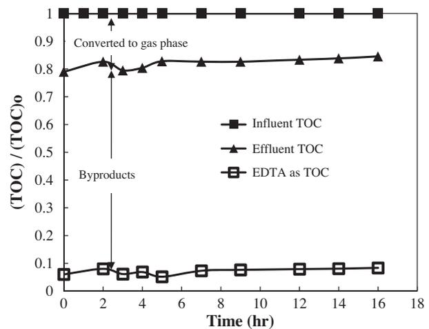
Fig. 8. TOC removal efficiencies for EDTA vs. time for influent, effluent TOC and EDTA as TOC with  $\text{TiO}_2$  under UV irradiation (both Cr(VI) and EDTA=0.001 M, pH=3.0, HRT=4.0 h with the aeration by air).
