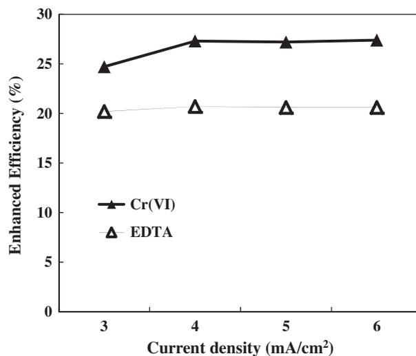
Fig. 3. A comparison of enhanced efficiencies for the (a) reduction of Cr(VI) and (b) oxidation of EDTA with  $\text{TiO}_2$  under UV irradiation with the ED system (both Cr(VI) and EDTA =  $0.001 \text{ M}$ ,  $\text{pH} = 3.0$ ,  $\text{HRT} = 4.0 \text{ h}$  with the aeration by air).
