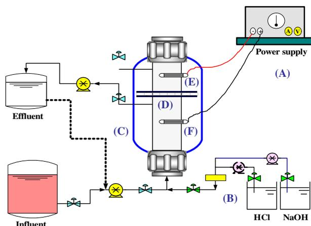
Fig. 1. Schematic diagram showing the photocatalytic reaction combining ionic exchange membrane processes: (A) DC power supply, (B) pH controller, (C) photocatalytic reactor, (D) CEM, (E) cathode and (F) anode.
