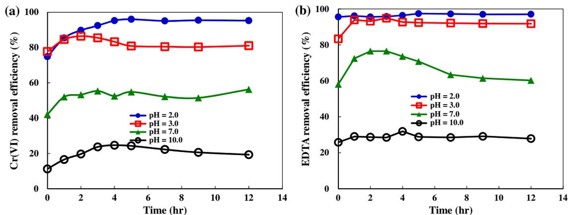
Fig. 4. A comparison of the removals of the (a) reduction of Cr(VI) and (b) oxidation of EDTA for different pHs with  $\text{TiO}_2$  under UV irradiation with the ED system (both Cr(VI) and EDTA = 0.001 M, HRT = 4.0 h with the aeration by air).
