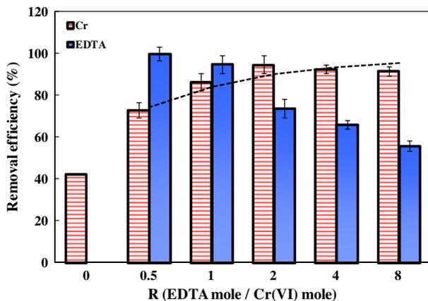
Fig. 6. Effects of the molar ratio of EDTA/Cr(VI) on their removal efficiencies with  $\text{TiO}_2$  under UV irradiation with the ED system (pH=3.0 and HRT=4.0 h with the aeration by air).
