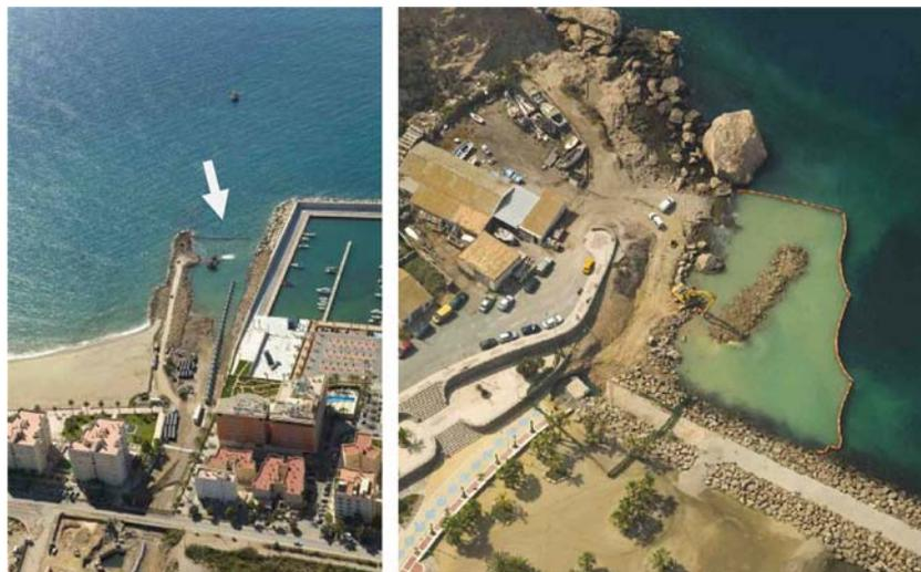
Fig. 5. Turbidity barriers installed at dry riverbed Cañarete (intake works) and El Charco (outfall works).
