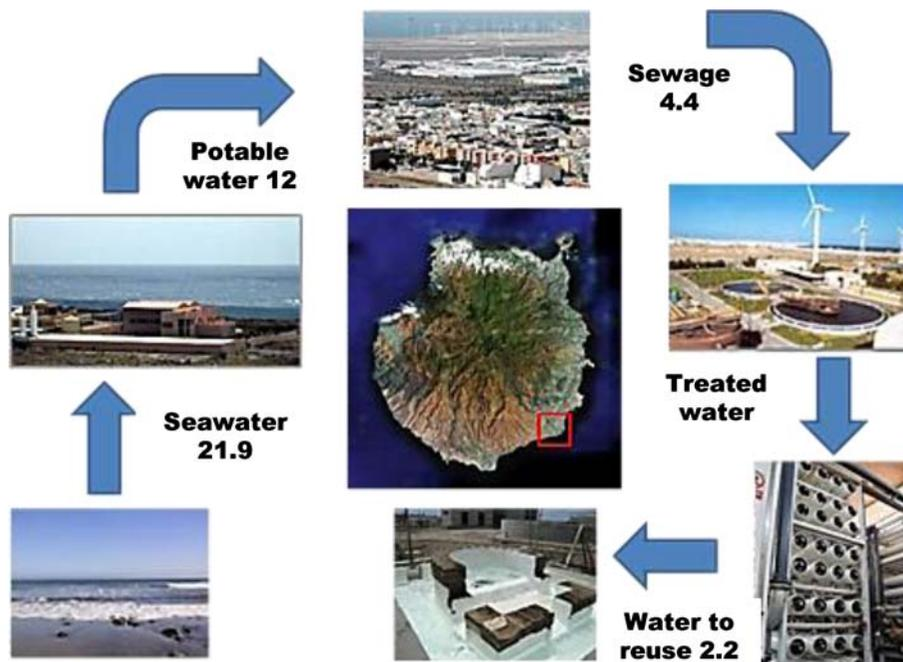
Fig. 3. Main scheme of the water cycle in the Mancomunidad del Sureste (Gran Canaria Island), and water balance in a typical year (hm<sup>3</sup>/y).
