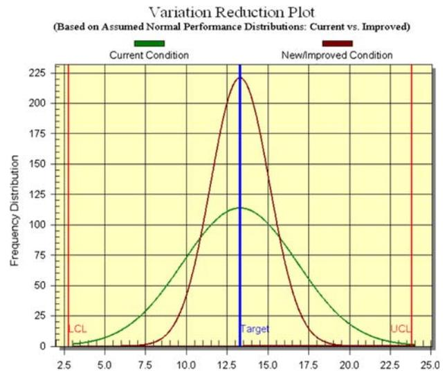
Fig. 4. Performance distribution of current and improved conditions for biogas production.
