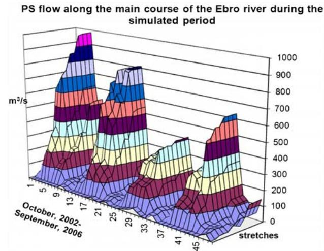
Fig. 4. PS flow along the main drain of the Ebro River.
