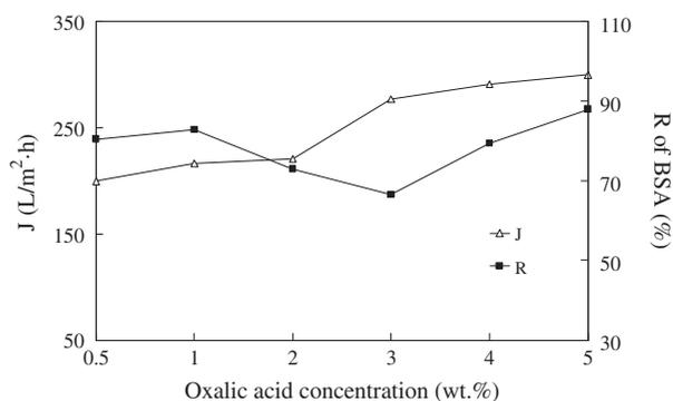
Fig. 8. Effects of oxalic acid concentrations on  $J$  and  $R$  of PES/3 wt.% Pluronic F127/oxalic acid ultrafiltration membranes.
