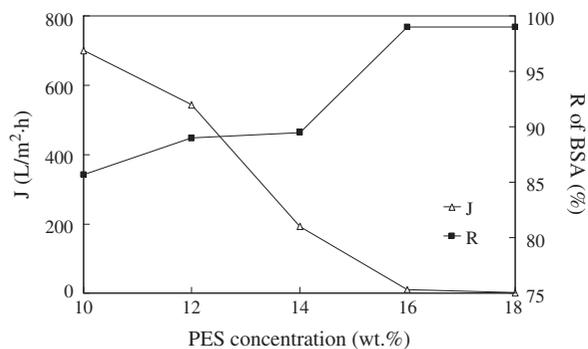
Fig. 4. Effects of PES concentrations on  $J$  and  $R$  of the neat PES ultrafiltration membrane.
