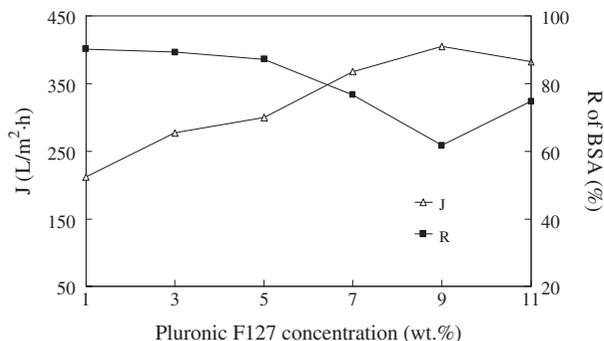
Fig. 6. Effects of Pluronic F127 concentrations on  $J$  and  $R$  of PES/ Pluronic F127 ultrafiltration membranes.
