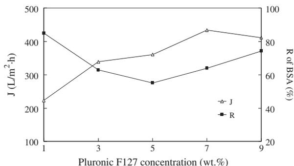
Fig. 12. Effects of Pluronic F127 concentrations on  $J$  and  $R$  of PES/Pluronic F127/4 wt.% PEG4000 ultrafiltration membranes.
