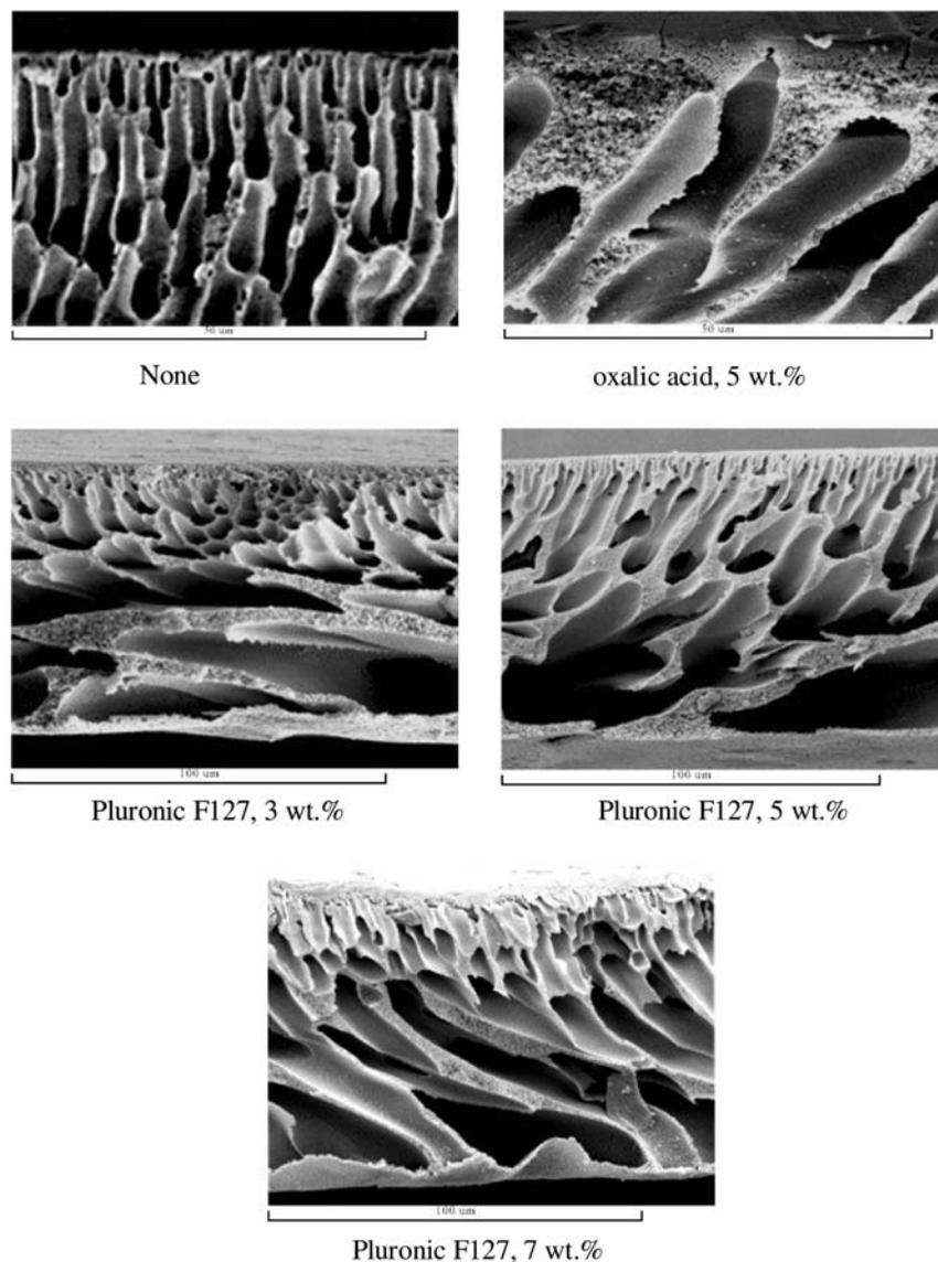
Fig. 7. Cross-section SEM micrographs of PES ultrafiltration membranes for different additives.
