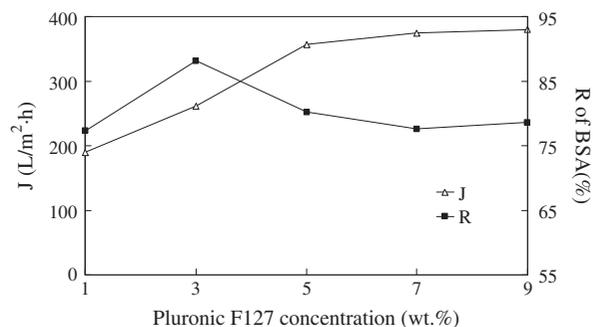
Fig. 9. Effects of Pluronic F127 concentrations on  $J$  and  $R$  of PES/Pluronic F127/1 wt.% oxalic acid ultrafiltration membranes.
