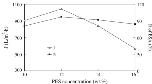
Fig. 5. Effects of PES concentrations on  $J$  and  $R$  of the PES/5 wt.% oxalic acid ultrafiltration membranes.
