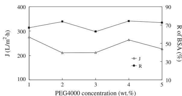
Fig. 11. Effects of PEG4000 concentrations on  $J$  and  $R$  of PES/3 wt.% Pluronic F127/PEG4000 ultrafiltration membranes.
