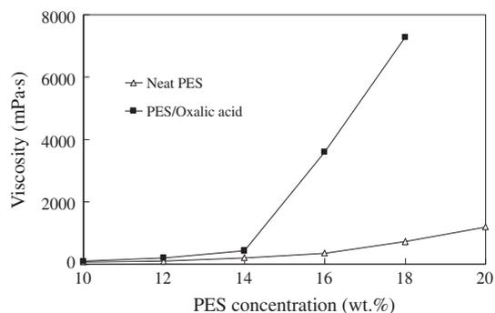
Fig. 3. Effects of PES concentrations on viscosity of different casting solutions (15°C).
