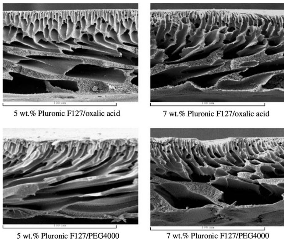
Fig. 10. Cross-section SEM micrographs of PES ultrafiltration membranes for different Pluronic F127 blended additives.
