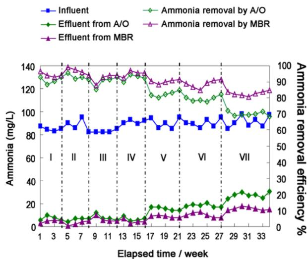
Fig. 3. Ammonia removal with different salinities.
