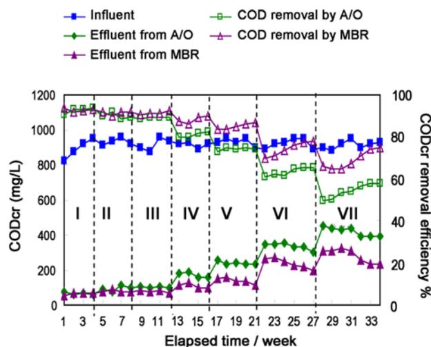
Fig. 2. COD removal with different salinities.
