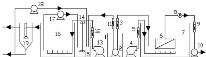
Fig. 1. Schematic diagram of submerged MBR and A/O processes. (1) Feed tank; (2) feed pump; (3,5,9,11,12) flowmeters; (4,13) air compressors; (6) membrane modules; (7) biological reactors; (9) pressure gauge; (10) suction pump; (14) stirrer; (15) anoxic tank; (16) aerobic tank; (17,18) recirculation pumps; (19) secondary settler.
